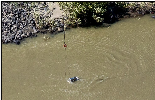
3. The helicopter pilot initiates the self releasing mechanism, causing the tank to invert and the salmon to be released.
