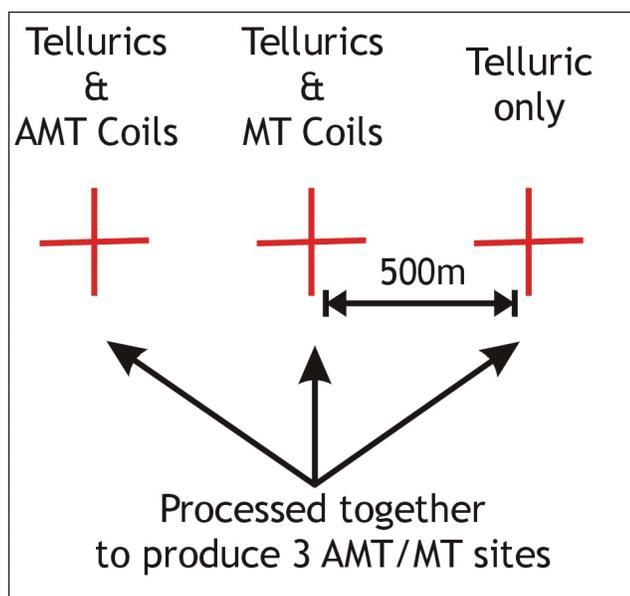
**Figure 2: Illustration of the site deployment and processing scheme developed to maximize the data quality and frequency range at each site.**
