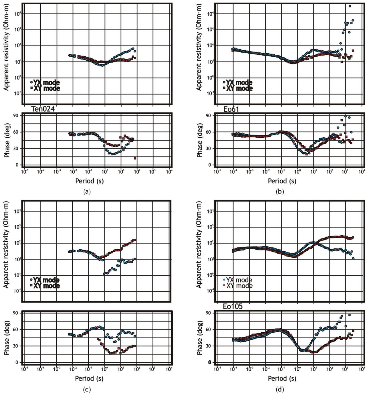
Figure 3: Examples of the improved data quality between the old Lithoprobe sites and the recent data acquisition in the Nechako Basin. The locations of the sites are shown in Figure 1, where (a) lithoprobe site ten24 and (b) Nechako site eo61 have the same position and (c) lithoprobe site ten21 and (d) Nechako site eo5 have the same position.
