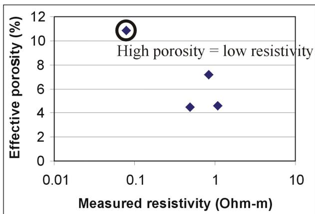
**Figure 8: Results of petrophysical analysis of several rock samples, showing the relationship between porosity and resistivity.**
