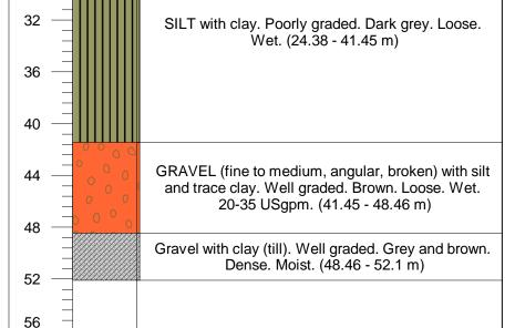
28 32 36 **Coated Bentonite** Pellets (39.83 -40 41.83 m) Schedule 40 PVC 10-slot screen (75 mm) (42.83 - 44.37 m) 48 10-20 Sand (52.1 -41.83 m) 52 56
