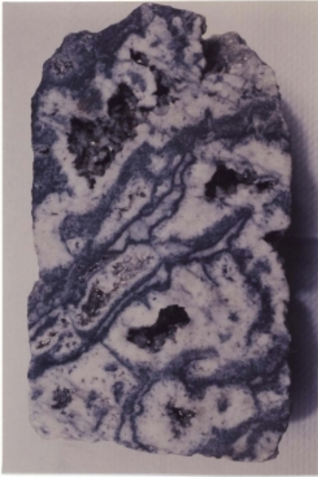
a. b-89-E/94-J-15 7429.8 ft. Upper Keg River Dolomite dark grey fabric preserving with some thin rims of light grey destructive replacive cement and coarse white cement infill following dissolution of stromatoporoid.
