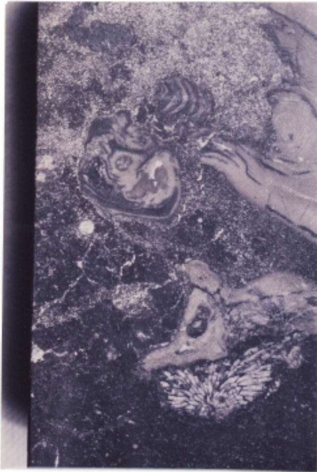
a. b-89-E/94-J-15 7348.5 ft. Upper Keg River Dendroid and massive stromatoporoid boundstone. Skeletal grainstone matrix pyrobitumen "saturated"; presumably degraded oil saturation.
