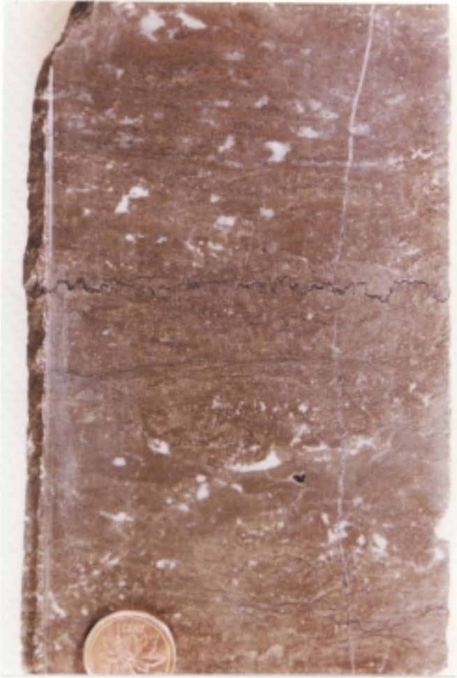
a. 10-7-99-8W6M 2272.30m Middle Slave Point Finely laminated peloid packstone and grainstone with fenestral fabric cemented by white sparry calcite.
