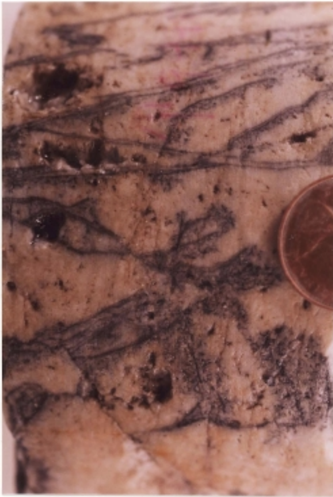
a. c-14-G/94-J-13 9987.5 ft. Chinchaga Coarse white megacrystalline dolomite composes eighty percent (80%) of the rock, but the cement overgrows a delicate web of earlier dolomite which appears to be the destructive replacive phase. This fabric might be inherited from anhydrite.
