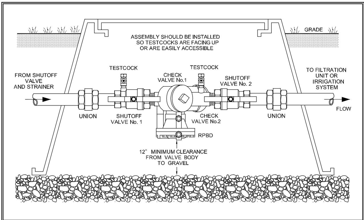
**Figure 4.4 DCVA or RPBD Installation - Below Ground**
