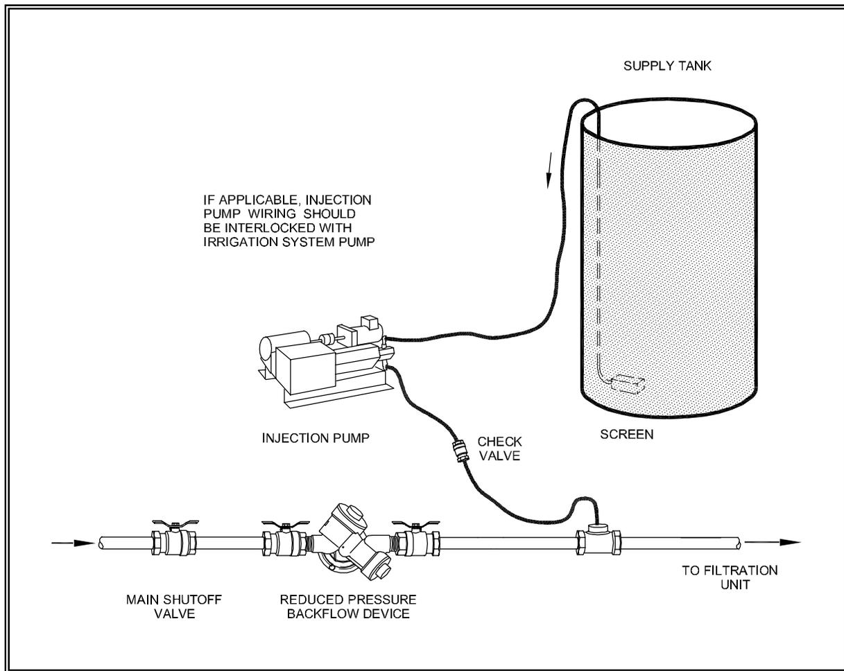
**Figure 6.4 Metering Injection Pump**
