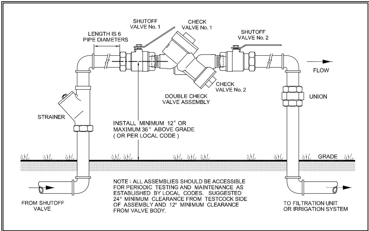
**Figure 4.3 DCVA or RPBD Installation - Above Ground**
