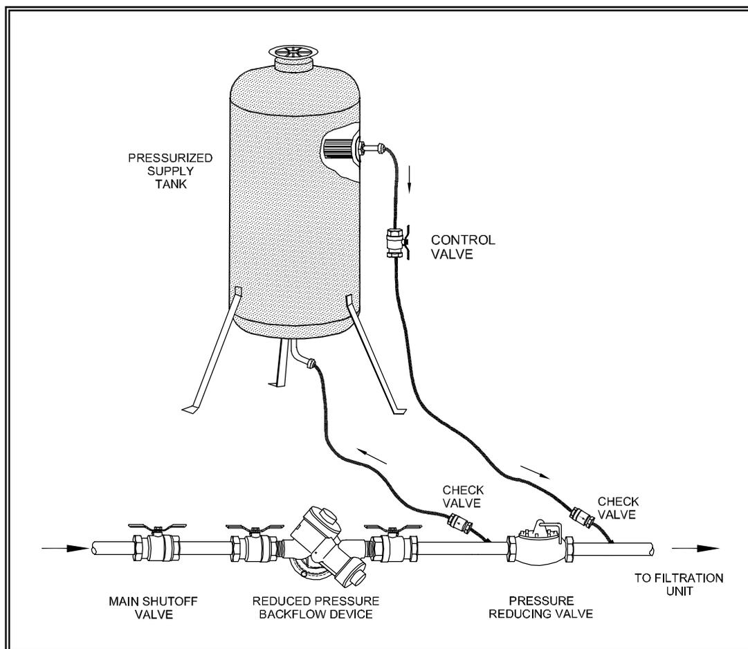
**Figure 6.2** Pressure Differential Injection System
