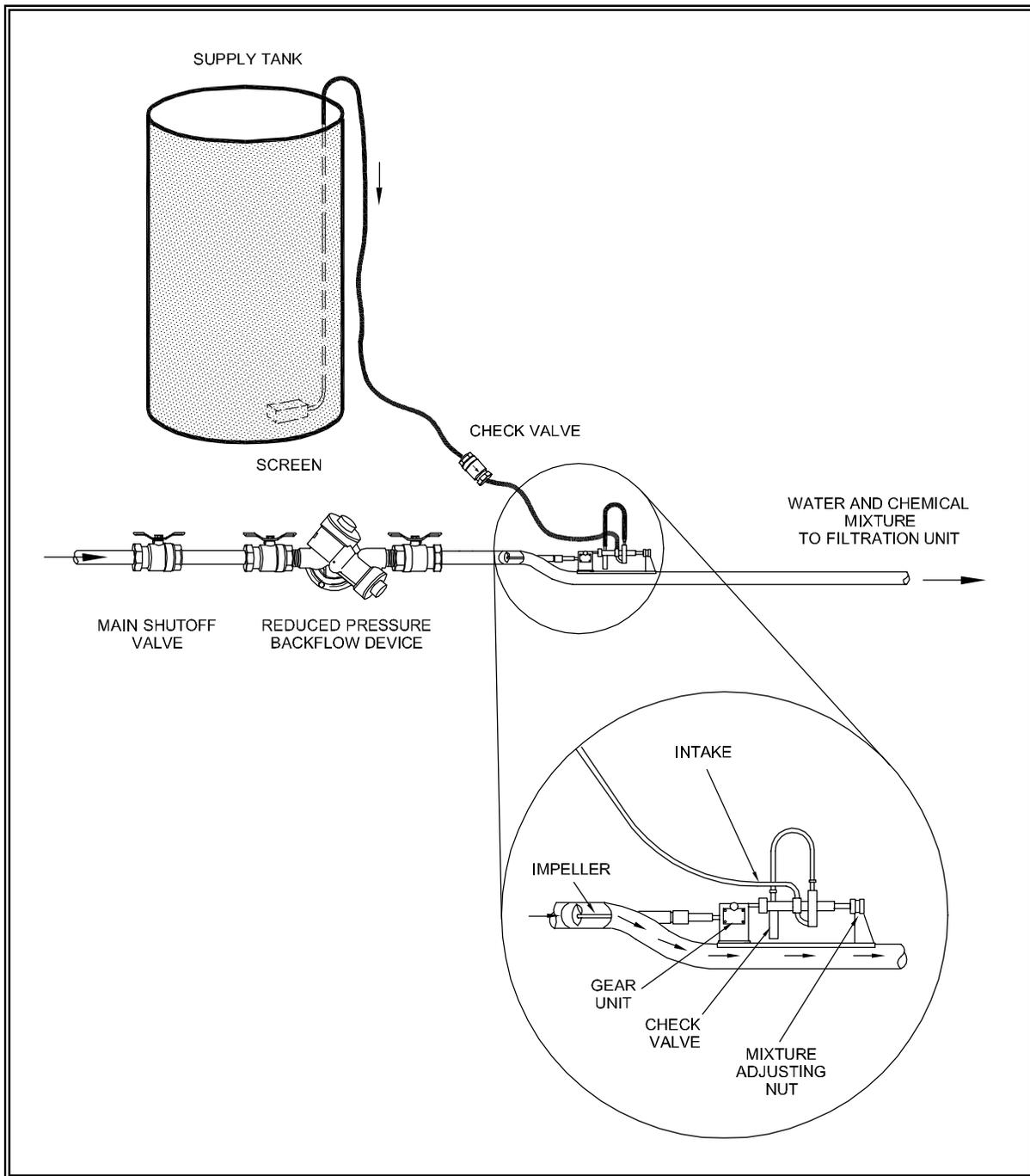
**Figure 6.5 Water Turbine Driven Injector**
