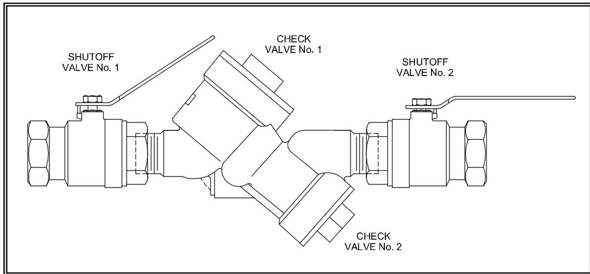
**Figure 4.1 Double Check Valve Assembly**
