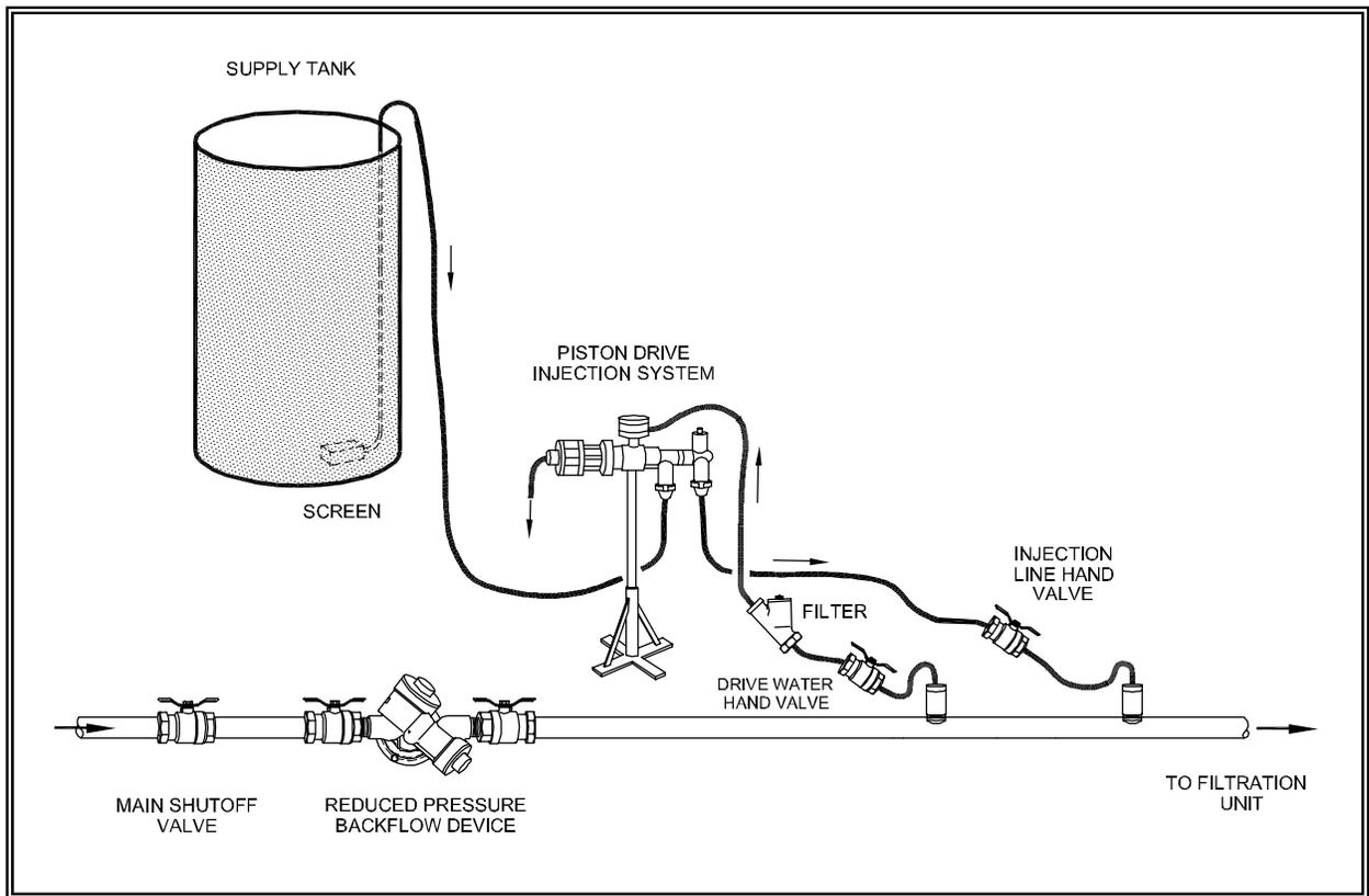
**Figure 6.6** **Piston Drive Injection System**
