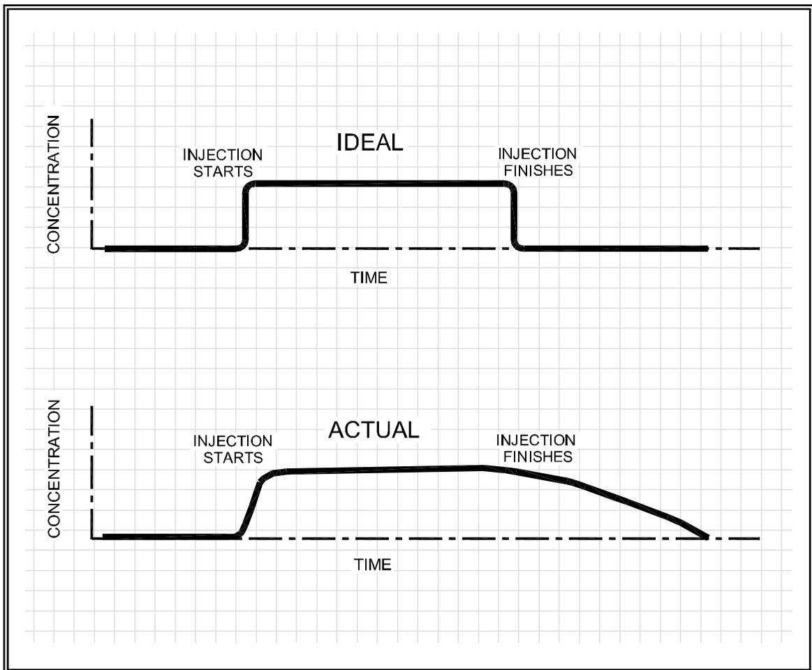
**Figure 3.1 Solute Dispersion Along Irrigation System**
