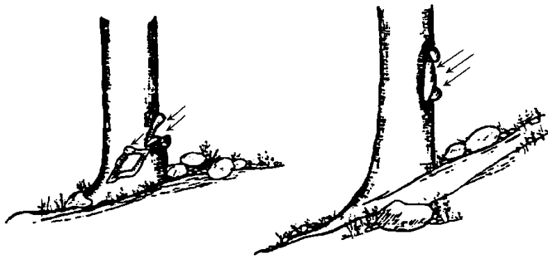
Figure A.20 Scars Caused by Rock Slides and Falling Rocks
