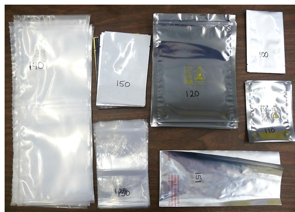
Figure 3. Seven bag types tested, including those currently used in the reforestation seed bank (140) and the 'zip-loc' type bags used in the seed lab for temporary storage (130).
