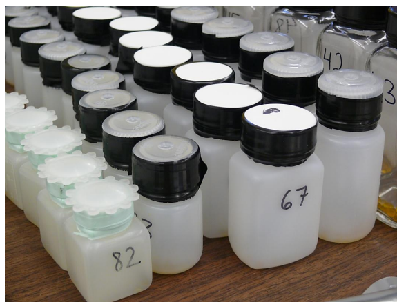
Figure 4. Method of sealing bottles involved tightening of lids and wrapping the join with either electrical tape or pipe joint tape (far left).
