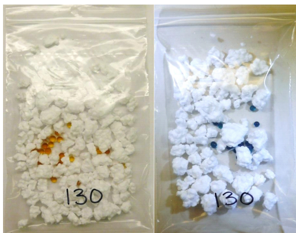
Figure 1. Example of indicator silica gel in 'zip-loc' type plastic bag showing before and after colour change from dry orange to humid green.
