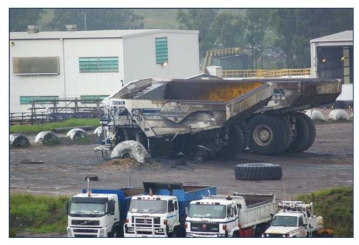
The tension created on the wheel had a force of approximately 270 kilonewtons (equivalent to 27,532 kilograms of weight). This force was strong enough to break 57 1-inch grade 10.9 bolts fastening the flange to the wheel.
