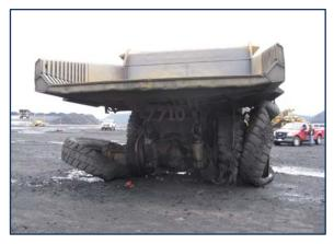
This haul truck was struck by lightning while parked at a dump. The truck's rear tires were blown off and propelled some 250 metres. All four rear tires were perforated and detached from the wheels of the truck.
