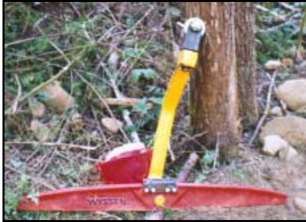
Figure 5.2-25 An intermediate support jack.
