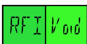
The Alco-Sensor FST® has been designed to be immune to RFI. Device has detected possible Radio Frequency Interference (RFI) at the time of the test and aborted the test process. Transmission on portable radios, in-car radios and cellular telephones is not advisable while conducting a test. Solution: Do not transmit on radios while conducting a test on the ASD.
