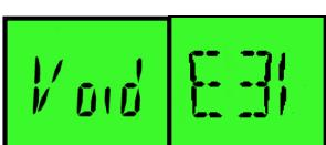
The result of the sample analysis is higher than the device maximum reading.
