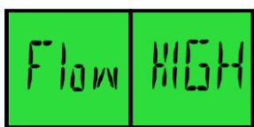
**Flow HIGH** indicates that the subject's breath flow exceeded the maximum allowable flow rate.
