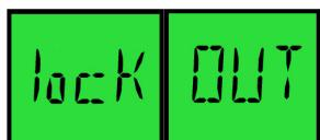
The device has not had a successful accuracy check within the designated lock out number of days. No further testing can be performed until a successful accuracy check has been conducted by a Qualified Technician trained in the calibration of the Alco-Sensor FST®.
