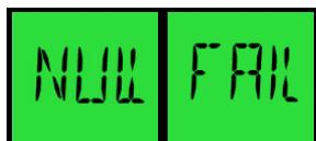
If the result of the blank test is not zero, a status message of NULL/FAIL will be generated. The test sequence will be aborted. Ensure that a new mouthpiece is used and that there is no ambient alcohol contamination. The result of the Blank Check must be "0" "WAIT" before the device will continue with the test sequence.
