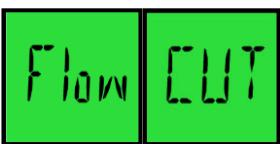
**Flow CUT** tells the operator that the subject provided enough breath flow to capture a sample, but their breath flow was stopped too abruptly or there has been an attempt to suck back the breath as the sample is being taken for analysis.
