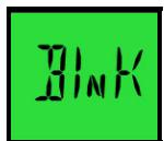
An air blank test (**BLINK**) is run automatically by the device to ensure that there is not alcohol present from a previous test.
