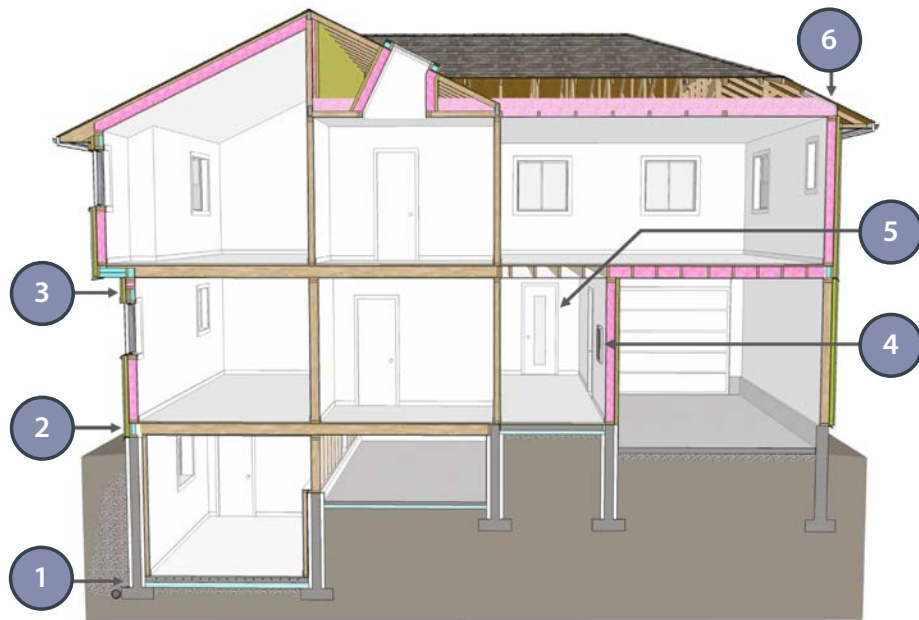
Figure 2: Typical Problem Areas for Insulation Continuity
