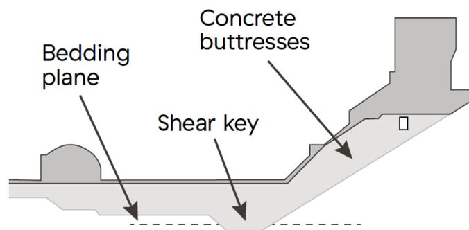
The original design for the Site C buttress extended the shear key about 35 metres below the bottom of the existing river channel and through what was, at the time, the deepest-known continuous bedding plane.
