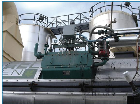
Water injection system on a drum mixing plant
