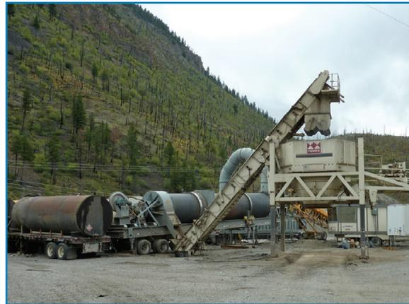
Typical portable asphalt plant
