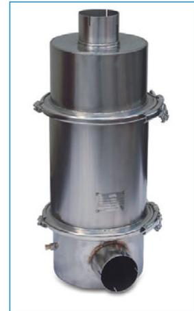
Diesel oxidation catalysts can reduce emissions of diesel particulate matter (PM) by 20 percent, hydrocarbons by 50 percent and carbon monoxide (CO) by approximately 40 percent, based on regular diesel fuel. They can be installed on off-road equipment and on diesel equipment that must operate within enclosed spaces (e.g. mines, buildings). A DOC can operate on virtually any engine on any duty cycle, and, as a passive device, is typically maintenance free.
