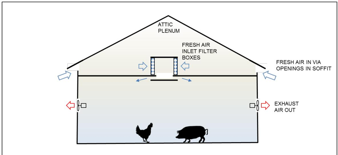
**Figure 44 - Intake Air Filtration Concept**
