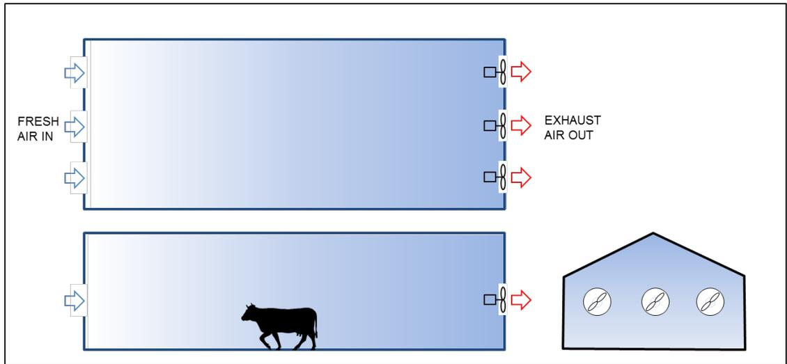
**Figure 10 – Forced Air Tunnel Ventilation Concept**
