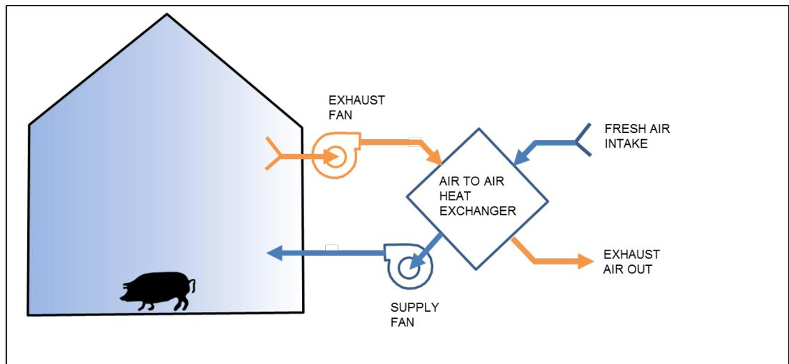
**Figure 29 - Air to Air Heat Recovery Concept**
