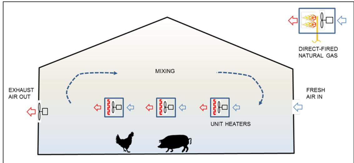
**Figure 21 - Unit Heaters Concept**
