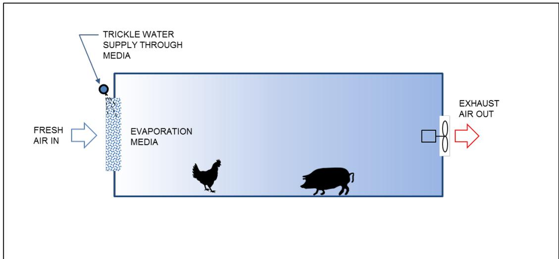
**Figure 27 – Direct Evaporative Cooling with Media Concept**
