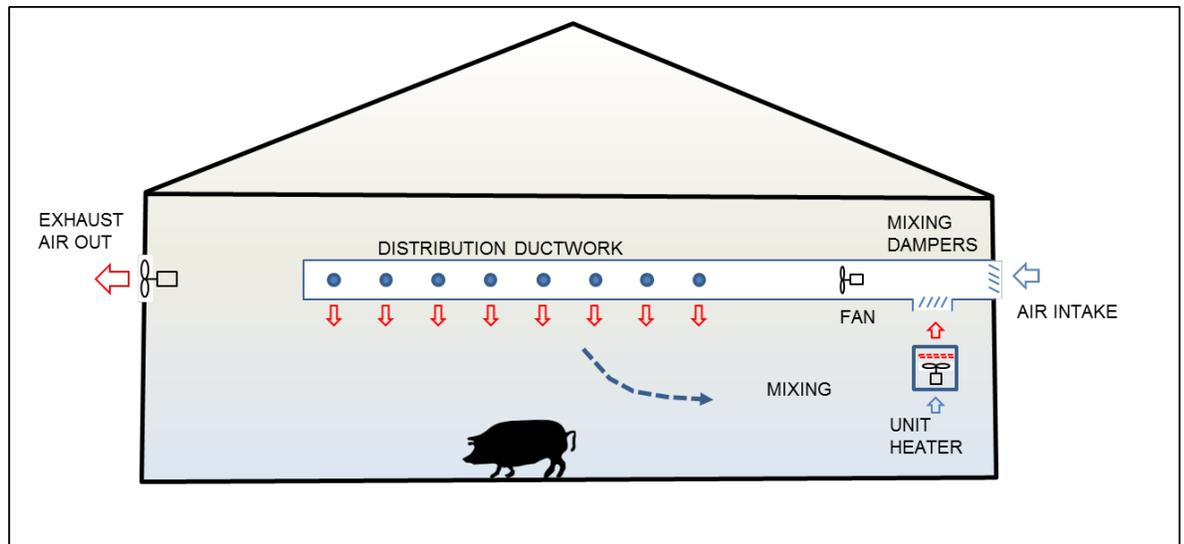
**Figure 13 - Combination Pressure/Exhaust System Concept**
