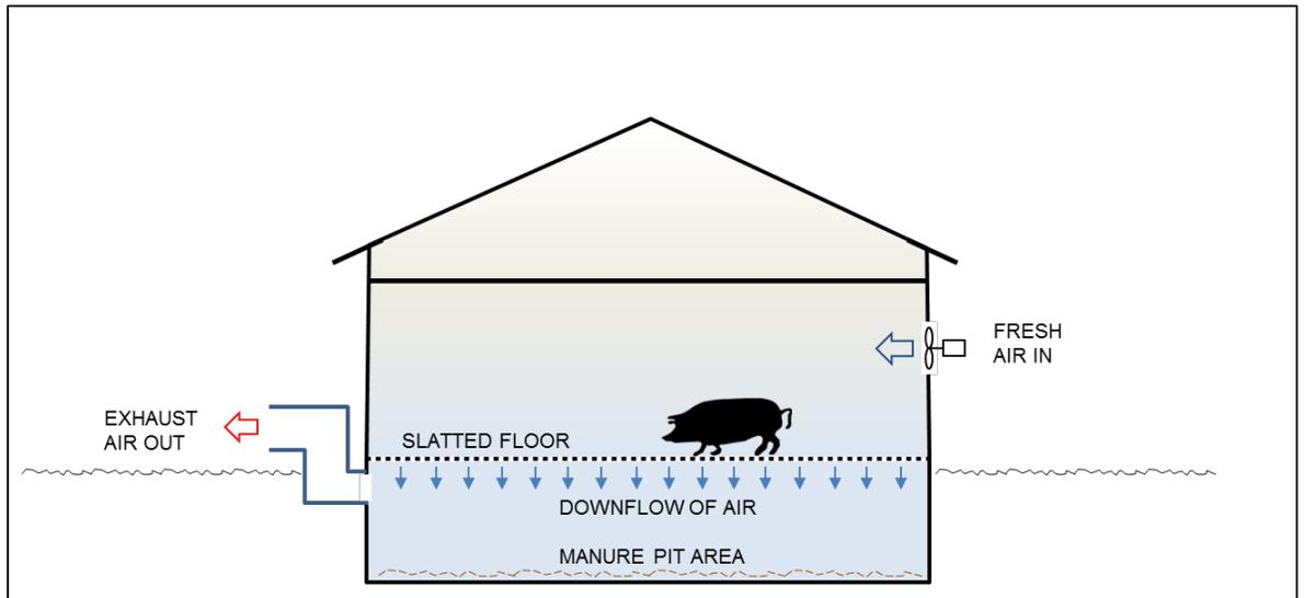
**Figure 16 - Positive Pressure Ventilation System Concept**
