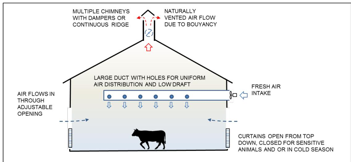
**Figure 15 - Distributed Forced Fresh Air with Natural Ventilation**
