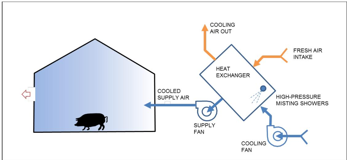
**Figure 28 - Evaporative Cooling in Forced Air Systems – Indirect – Concept**
