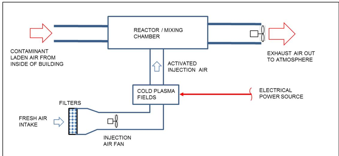
**Figure 48 - Non-Thermal Plasma for Exhaust Air Odour Abatement Concept**
