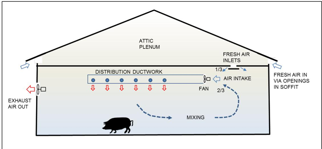
**Figure 24 - Ducted Recirculation System Concept**
