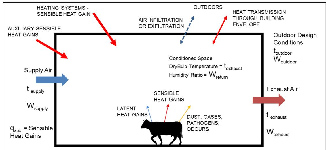
Figure 51 - Energy and Mass Balance
