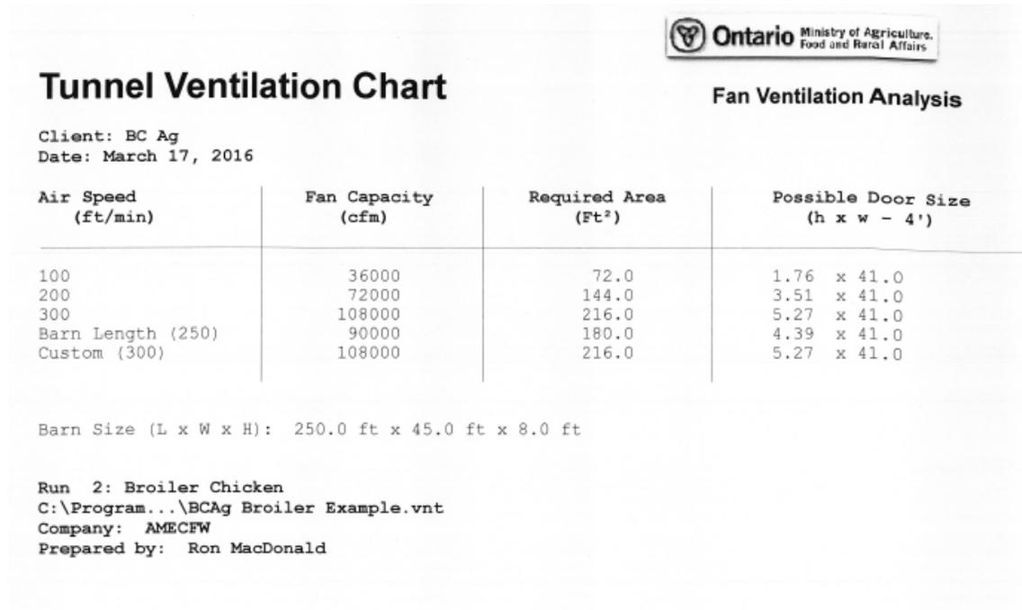
**Figure 60 - Tunnel Ventilation Chart**
