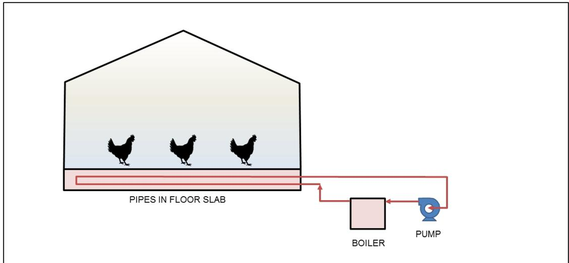
**Figure 18 - In-Floor Heating Concept**
