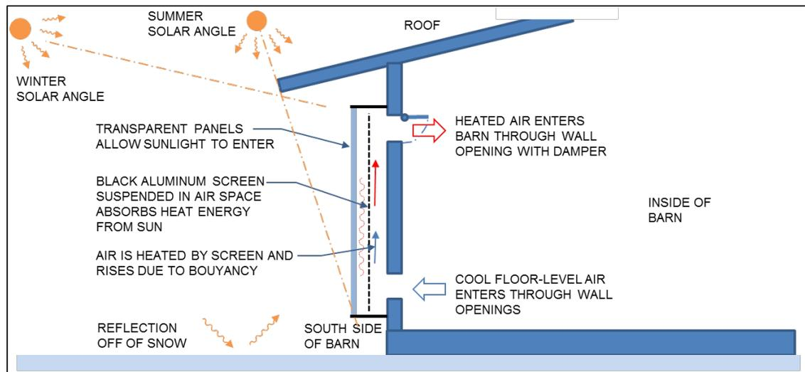
**Figure 35 - Passive Solar Air Heater Concept**
