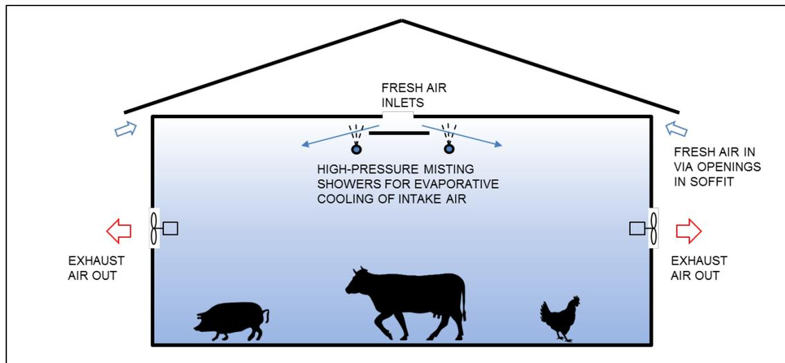
**Figure 26 - Evaporative Cooling with Direct High-Pressure Misting Concept**
