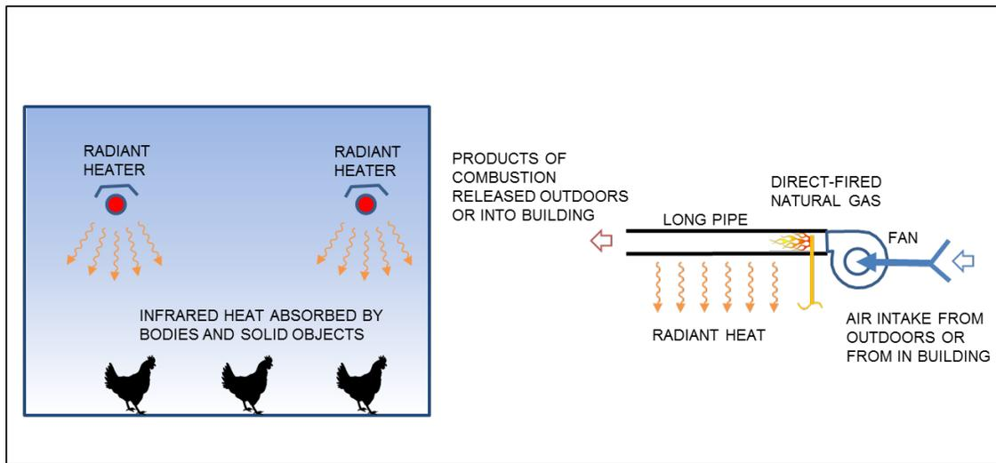
**Figure 19 - Gas-Fired Radiant Heating Concept**
