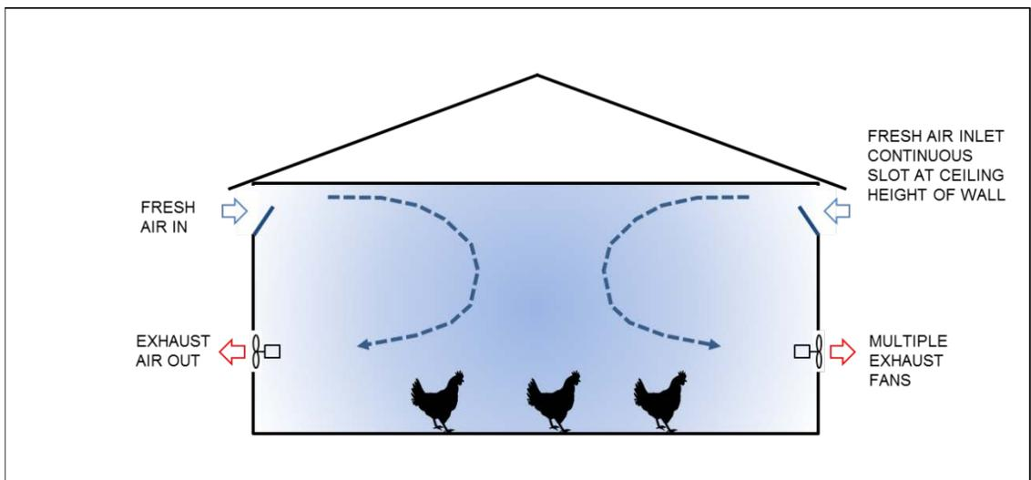
Figure 7 - Exhaust Ventilation (inlets both sides) System Concept
