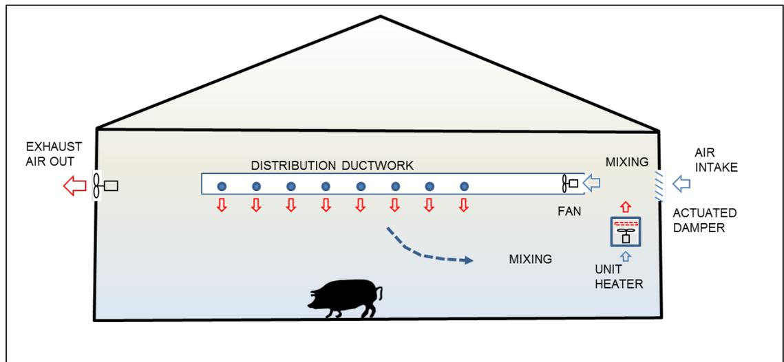
**Figure 9 - Exhaust Ventilation with Ducted Recirculation System Concept**
