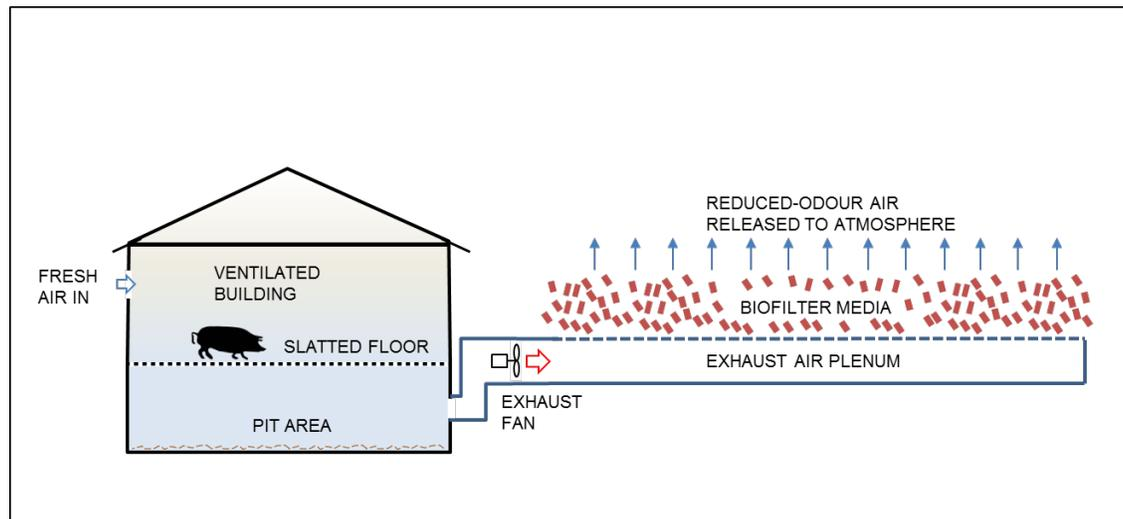
**Figure 45 - Biofiltration on Building Exhaust Concept**
