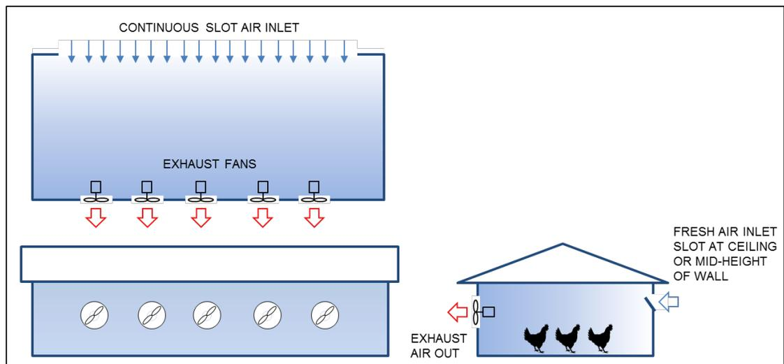
**Figure 8 - Exhaust Ventilation (Cross-Ventilation) System Concept**
