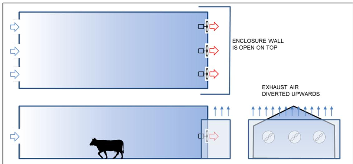
**Figure 49 - Windbreak Wall Concept**
