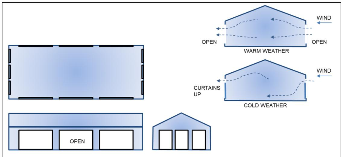
**Figure 4 - Natural Ventilation with Side Walls and End Walls Concept**
