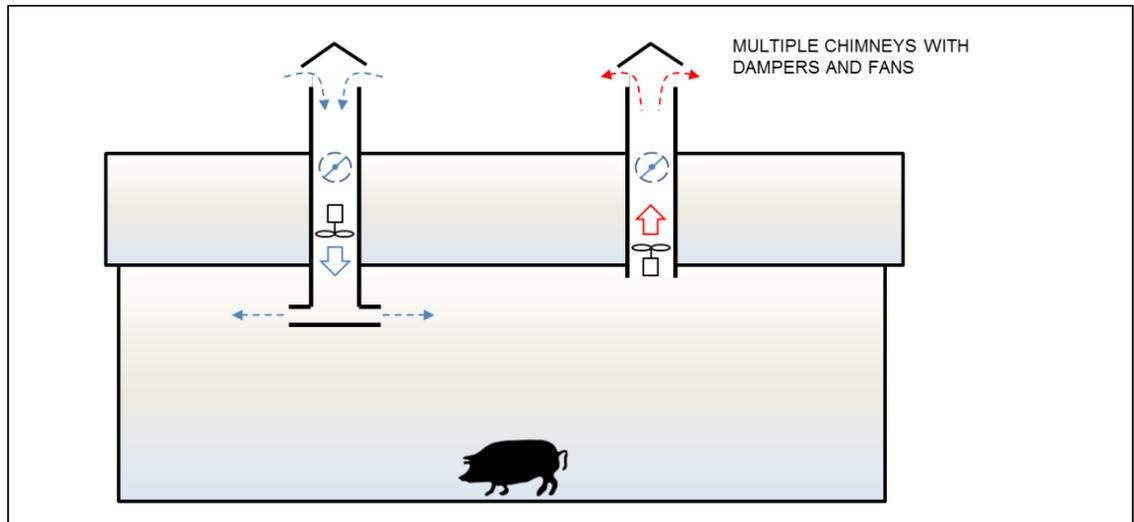
**Figure 14 - Forced Air – Neutral Pressure System Concept**
