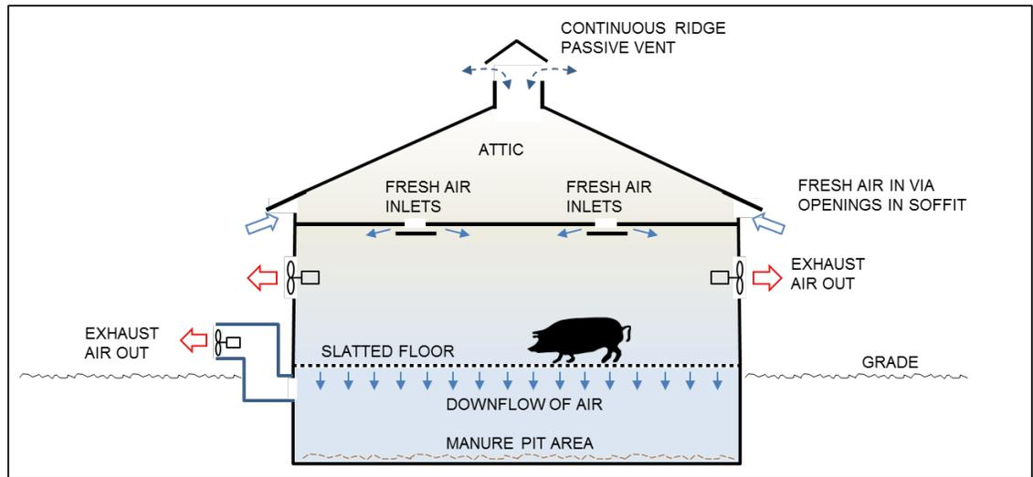
**Figure 12 - Attic Inlet Plenum with Pit and Side Wall Exhaust Fans Concept**
