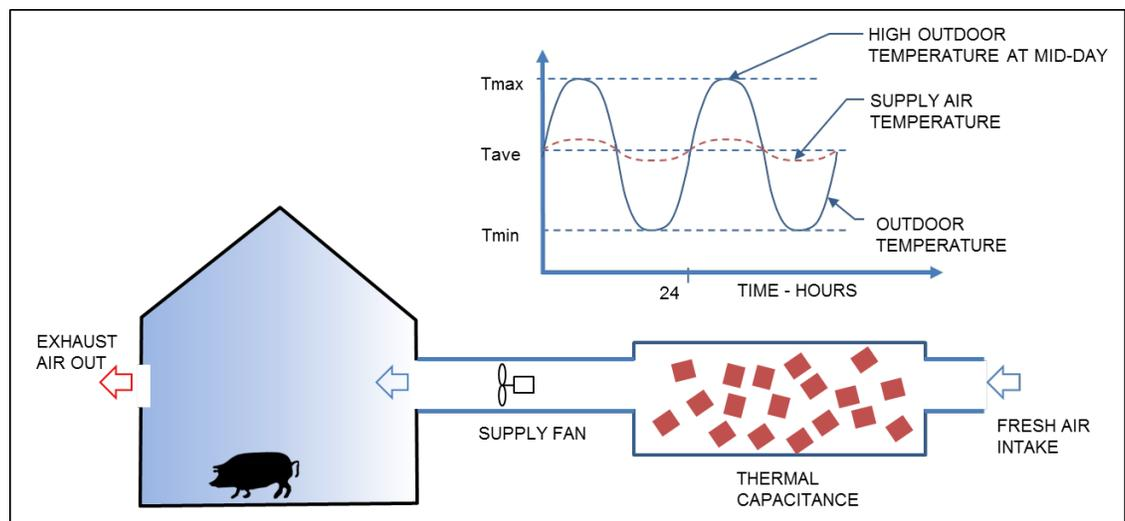
**Figure 31 - External Thermal Capacitance Concept**
