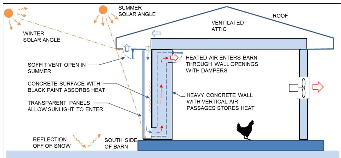
**Figure 34 – Solar Ventilation Wall with Heat Storage Concept**
