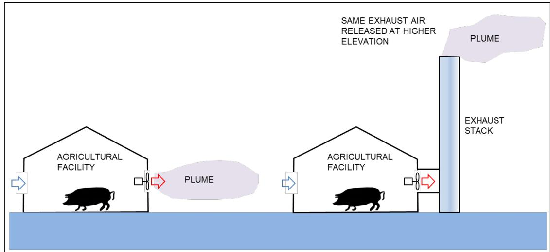
**Figure 50 - Exhaust Stack Concept**
