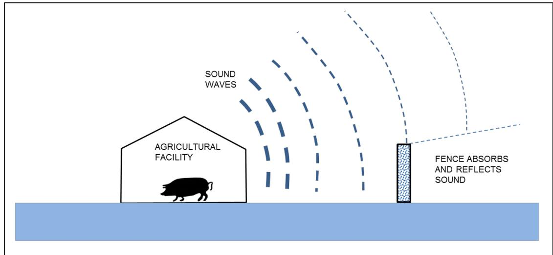
**Figure 38 – Noise Barrier Fence Concept**
