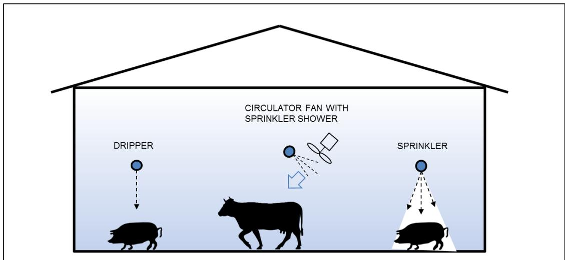
**Figure 25 - Cooling with Low-Pressure Water Sprinklers or Drippers**
