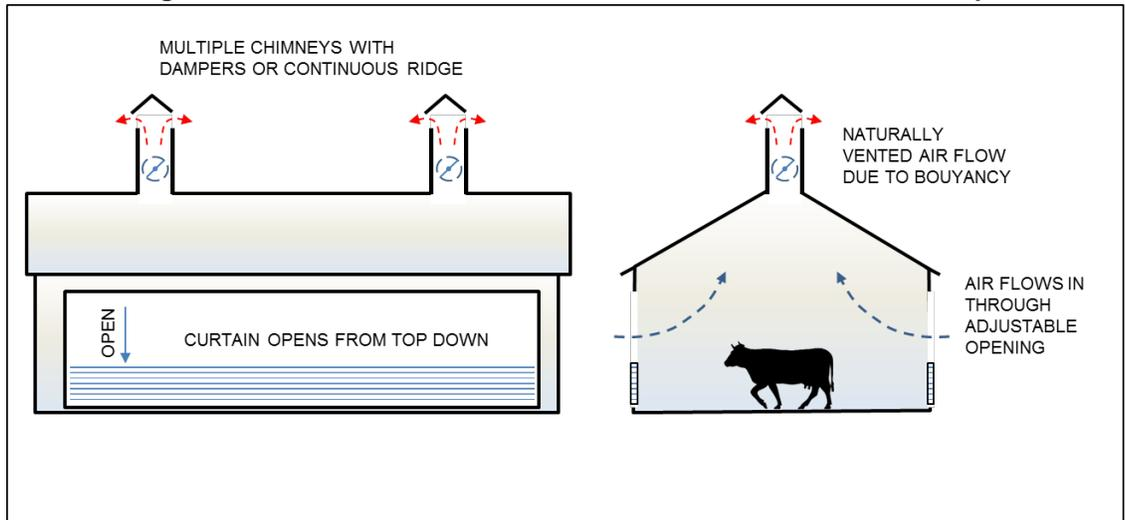
**Figure 5 - Natural Ventilation with Chimneys or Continuous Ridges Concept**
