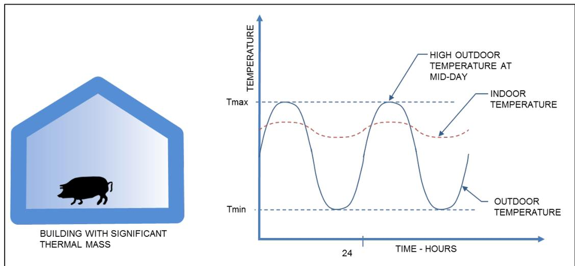
**Figure 30 - Building Thermal Capacitance Concept**
