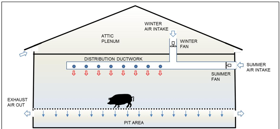
**Figure 17 - Ducted Positive Pressure System Concept**
