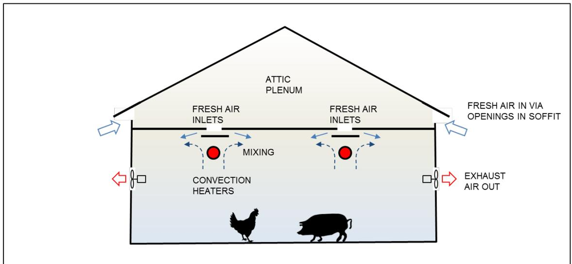
**Figure 20 - Convective Heating Concept**
