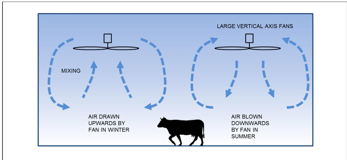
**Figure 23 - Down Draft High Volume Low-Speed (HVLS) Circulation System Concept**
