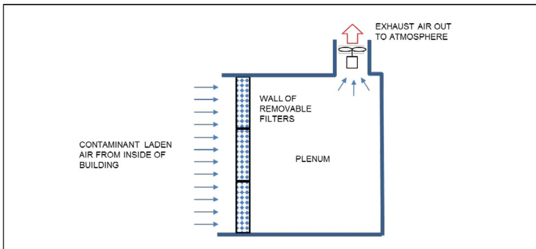
**Figure 43 - Air Filtration for Exhaust Air Cleaning Concept**
