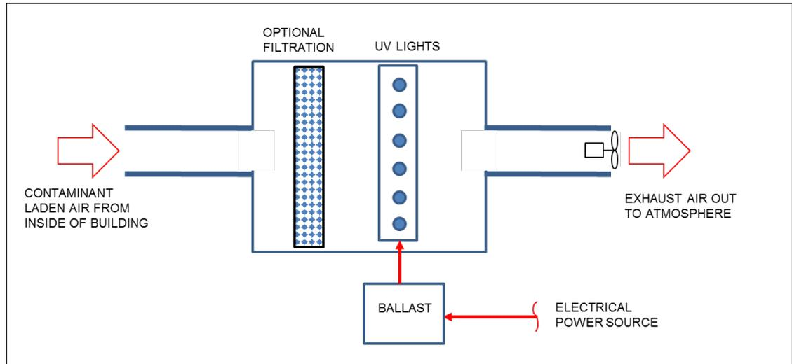
**Figure 47 - Ultraviolet Light for Exhaust Air Cleaning Concept**
