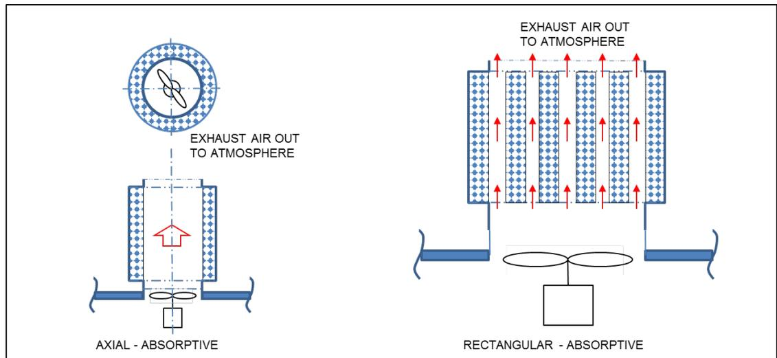
**Figure 42 - Ducted Sound Attenuators Concept**
