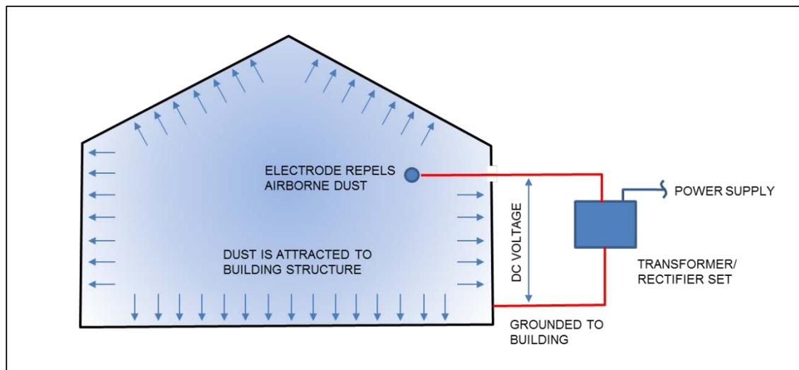
**Figure 41 - Building Electrostatic Charge for Dust Abatement Concept**
