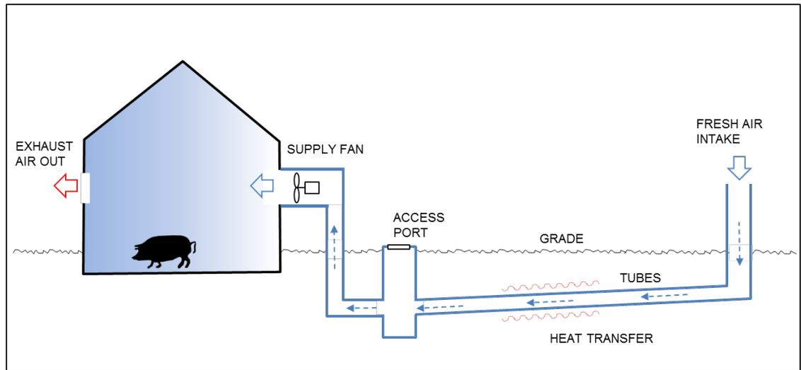
**Figure 32 - Earth Tube System Concept**
