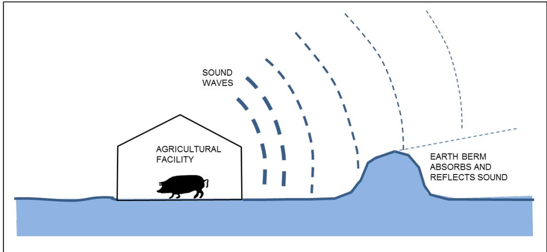
**Figure 37 - Noise Control Earth Berm Concept**
