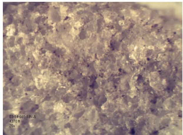
Close-up view at 20X magnification of a single chip. Fair to good textural relief indicates good intergranular porosity. Only minor detrital material is present among the predominant quartz grains.
