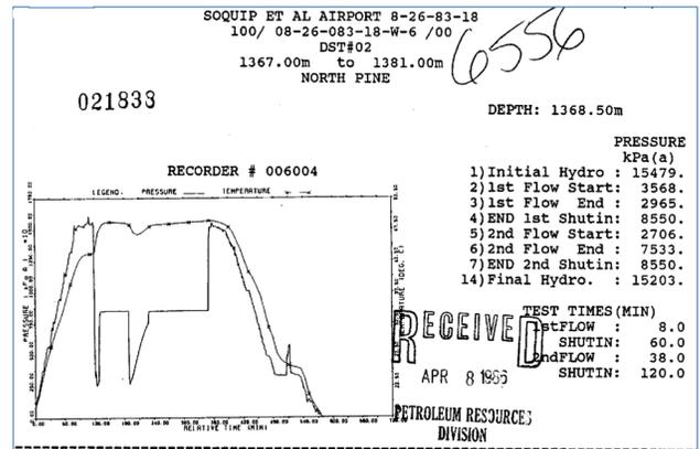
Figure 8. DST #2 at location 8-26-83-18W6. Very good to excellent permeability is displayed by almost immediate stabilization upon shut-ins. Oil (200 m) and water (100 m) were recovered.
