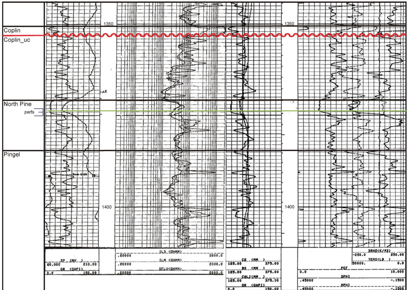
Figure 5. Location 8-26-83-18W6 induction and neutron-density logs: Neutron-density crossover in the North Pine indicates gas. This gas component has been important for the efficient 50% recovery rate of the pool. A gas-oil contact is at 1373 m measured depth (-706 m mean sea level).
