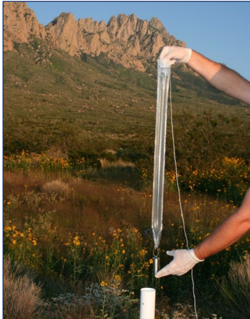
Figure 2-13 Example of a no-purge method: HydraSleeve.
