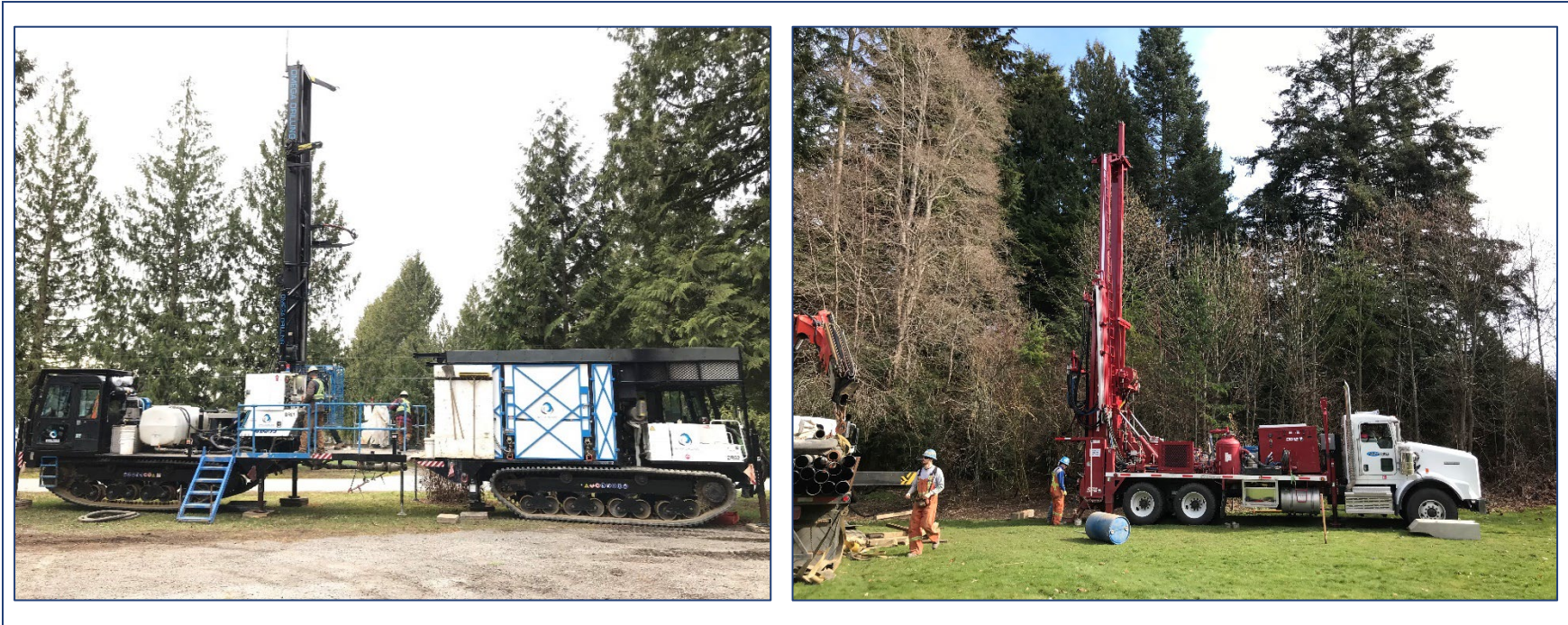
Figure 5-4 Examples of sonic (left) and dual rotary (right) drilling equipment.
