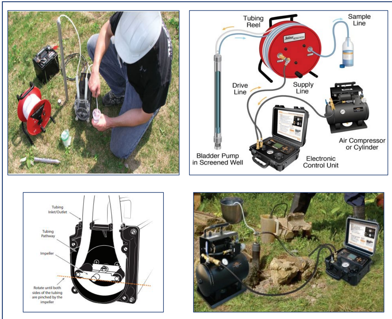
Figure 2-12 Examples of low-flow sampling instrumentation, such as peristaltic pump sampling from a drive-point piezometer (top left), the peri-pump operating mechanism (bottom left), bladder pump (top right) and bladder pump in operation (bottom right).
