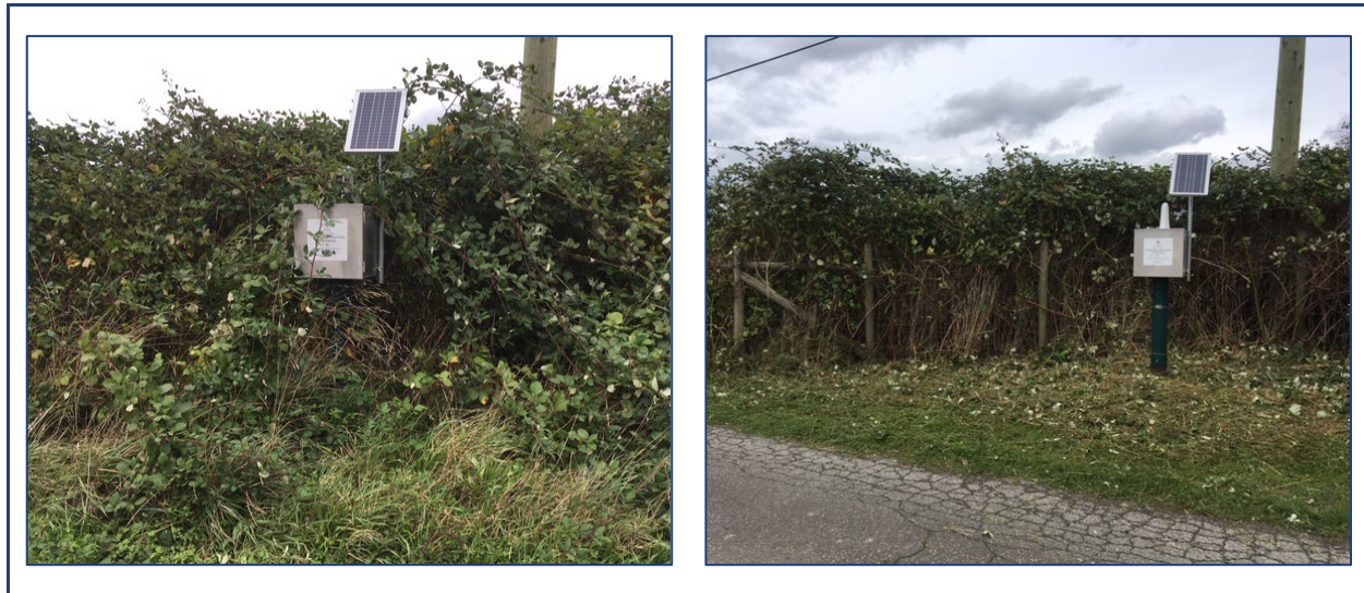
Figure 2-15 A Provincial Observation Well with excessive vegetation build-up (left) and after brush-clearing (right).
