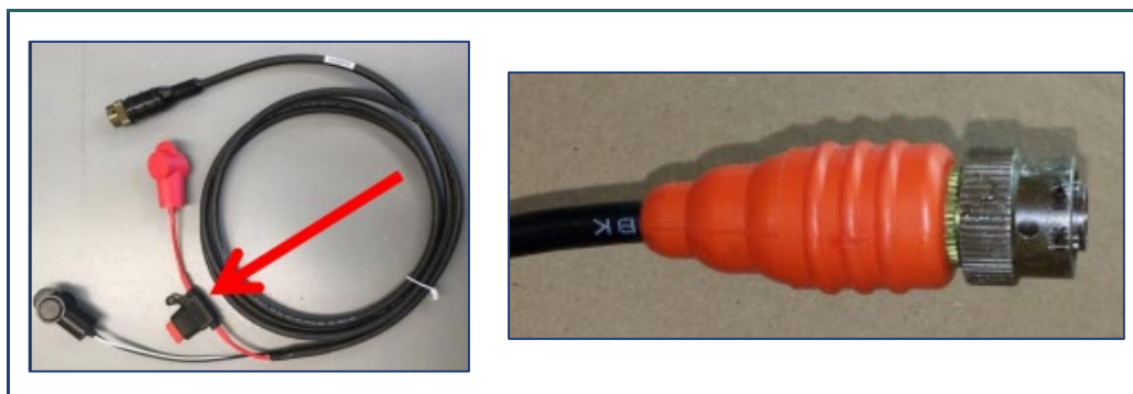
Figure A2-2.2 Components of an FTS datalogger power cable.
