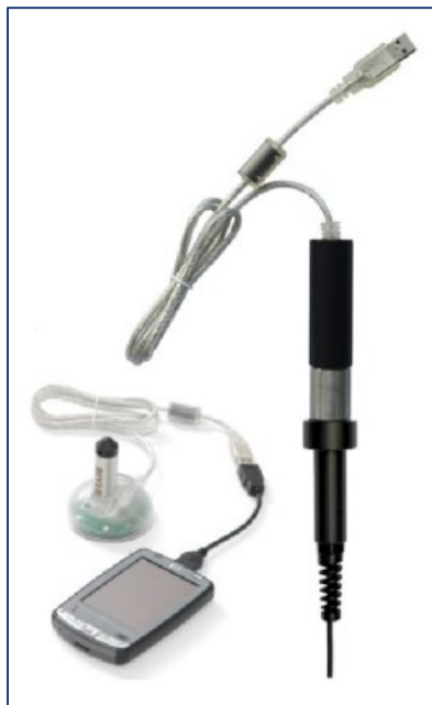
Figure A2-4.2 Van Essen optical reader (left) and direct-read cable (right).
