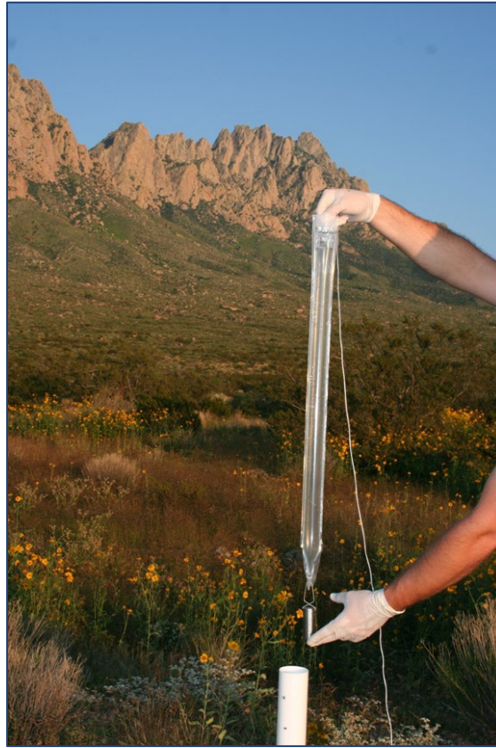
Figure A3-1.6 Example of a no-purge method: HydraSleeve.
