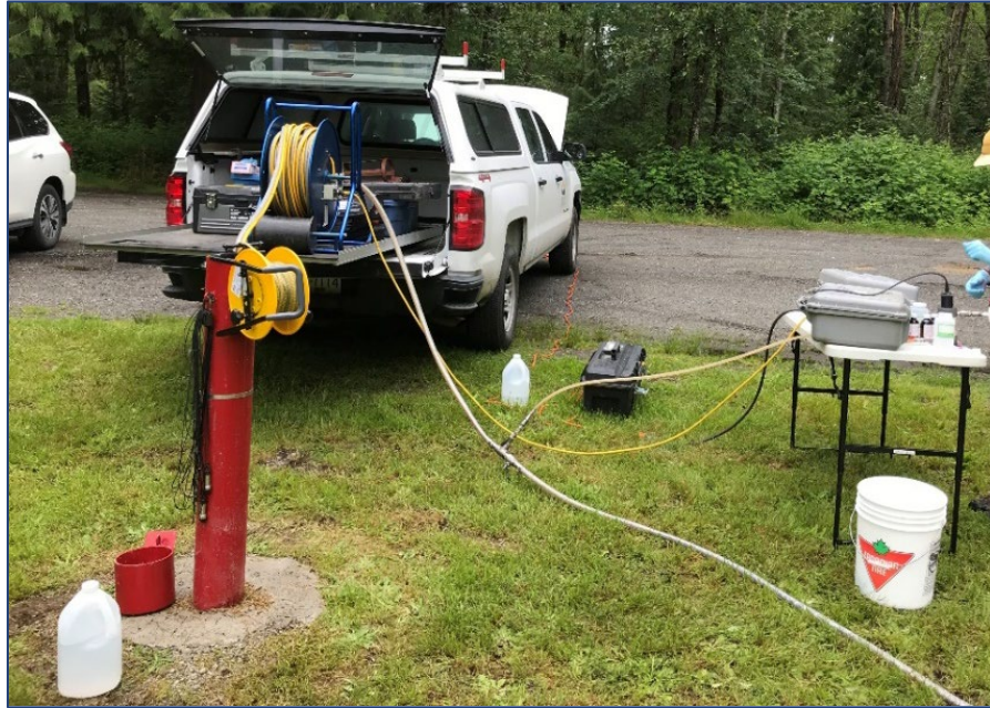
Figure A3-1.2 Typical groundwater purge sampling set-up.
