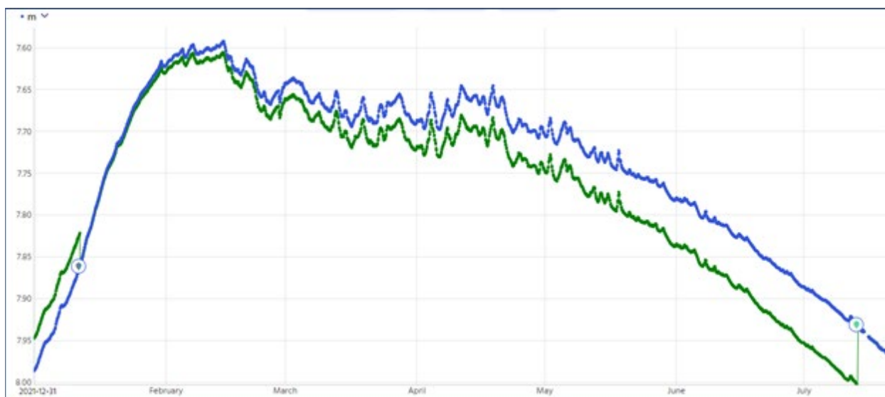
Figure 4-8 Example of drift corrections aligning with Field Visits in Aquarius. Green is raw data and blue is corrected data, with encircled pins being Field Visits.
