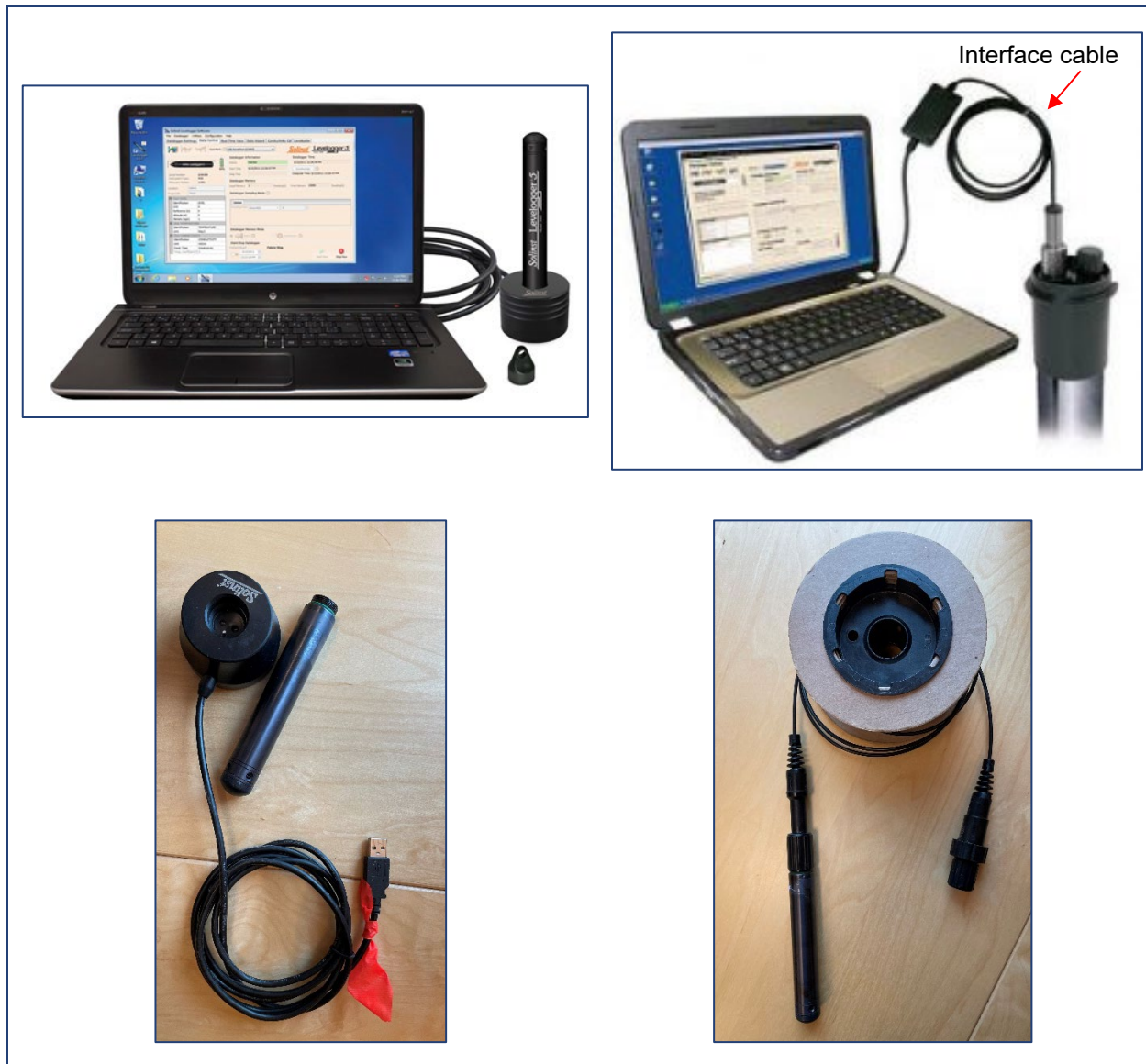
Figure A2-4.1 Solinst optical reader (left) and direct-read cable (right).
