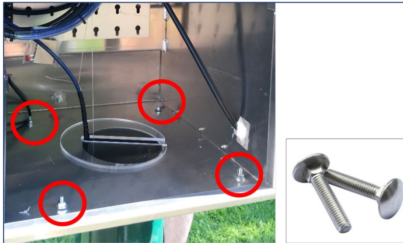
Figure 3-6 Illustration of carriage bolt alignment within the wellhead cabinet.
