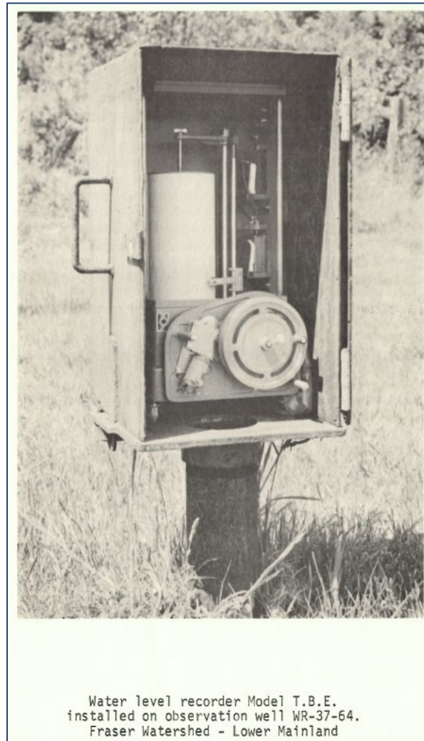
Figure 1-1 Image of a Stevens Chart Recorder at one of the first Provincial Observation Wells.
