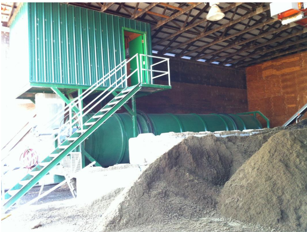
Figure 3. The solid output of a Bedding Recovery System.
