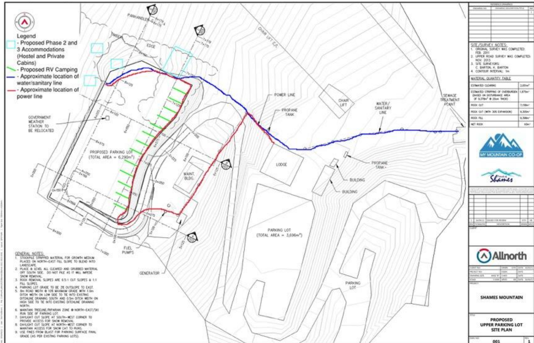
Drawing 1. Conceptual plan for new parking lot area and On-Hill Accommodation Phase I: RV camping for Shames Mountain Ski Area.
