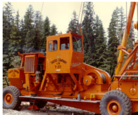
A newly acquired Tahsis company Sparmatic yarder in July 1963, manufactured by Tyee Machinery Ltd. These 120 foot steel towers were new technology at the time and replaced wooden spar trees, dramatically changing coastal logging practices.
