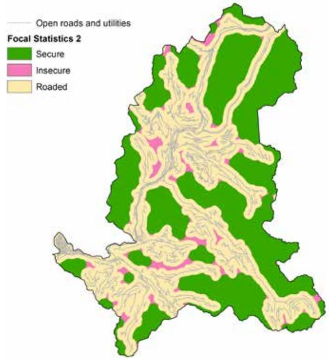
Fig.4d. Focal Statistics 2 'ballooning' to add adjacent Secure areas
