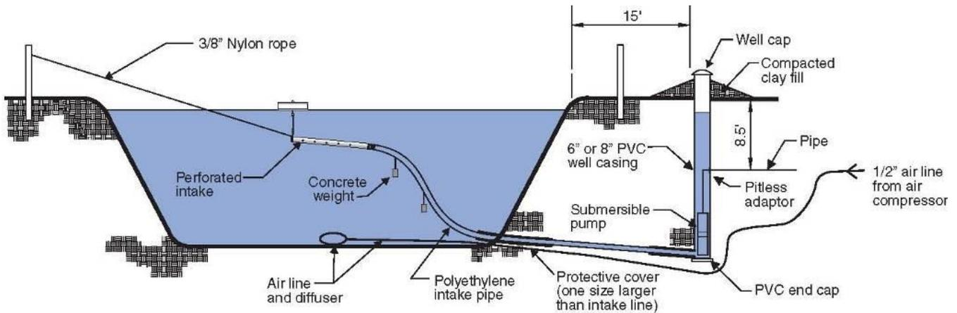
**Figure 18 Submersible Pump and Intake System**
