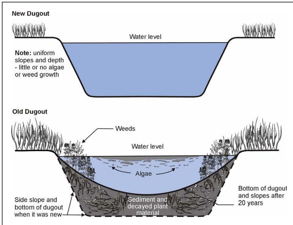
**Figure 12** New vs. Old Reservoir Cross Sections
