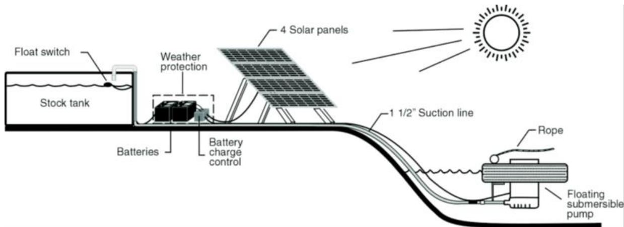
**Figure 20 Solar Watering System**
