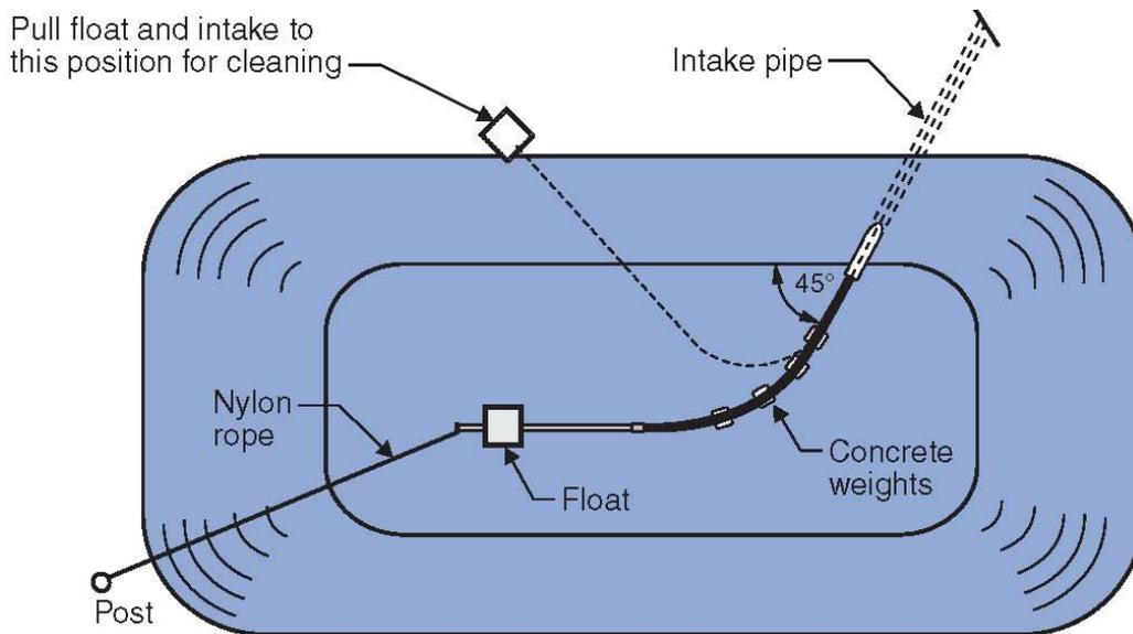
**Figure 19 Plan View of Intake System**
