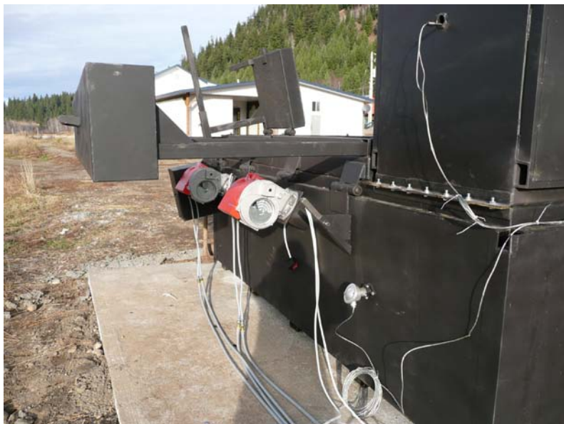
Photo 2. Side view of incinerator showing two primary chamber burners.
