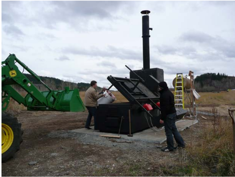
Photo 3. Manually loading incinerator through top-loading door.
