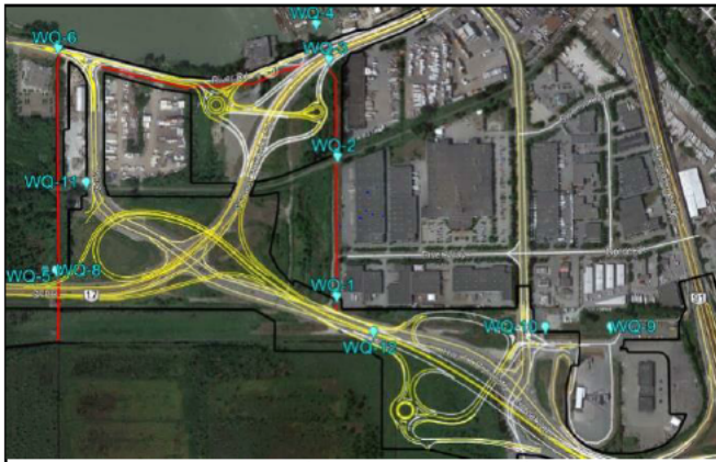
Figure 1: Baseline water sampling locations, WQ-7 is grouped with WQ-5 and WQ-8. Samples were only collected at locations where work is being done.
