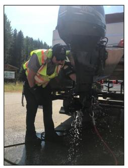
Engine flush being performed by inspectors at the Yahk inspection station as part of the decontamination of a high risk pontoon boat.
