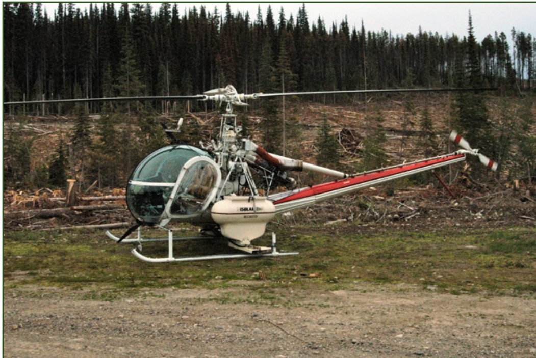
Hiller 12E helicopter equipped with spreader for verbenone application.
