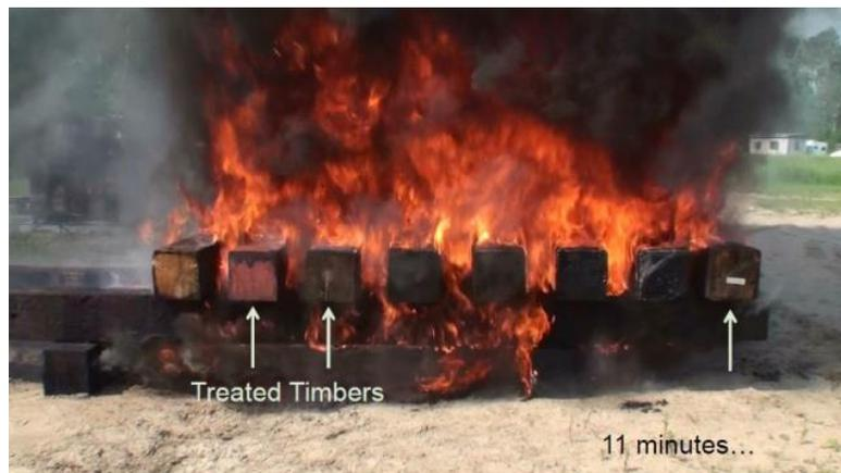
Figure 4. FPInnovations bridge timber treatment ignition test (Razim 2020).
