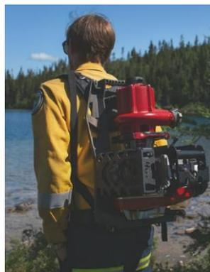
Figure 3. The lightweight MK III pump allows for easy transport into the forest.
