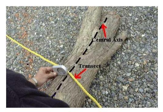
Figure 2. The clinometer is used to measure the angle the CWD makes from the horizontal.
