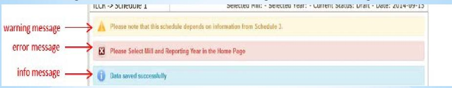
Error, warning, and info messages will display at the top left of each screen. Multiple messages can be displayed on the screen at once.
