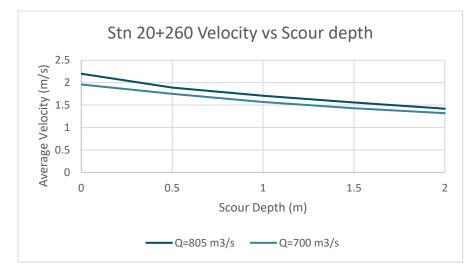
Figure 4: Existing Baxter Bridge Flow Velocities for Various Scour Depths
