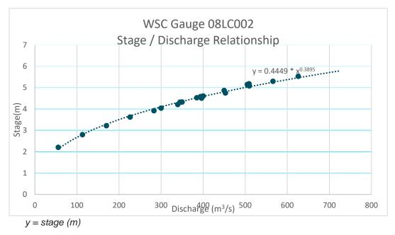
Figure 2: Stage / Discharge Relationship for WSC Gauge 08LC002
