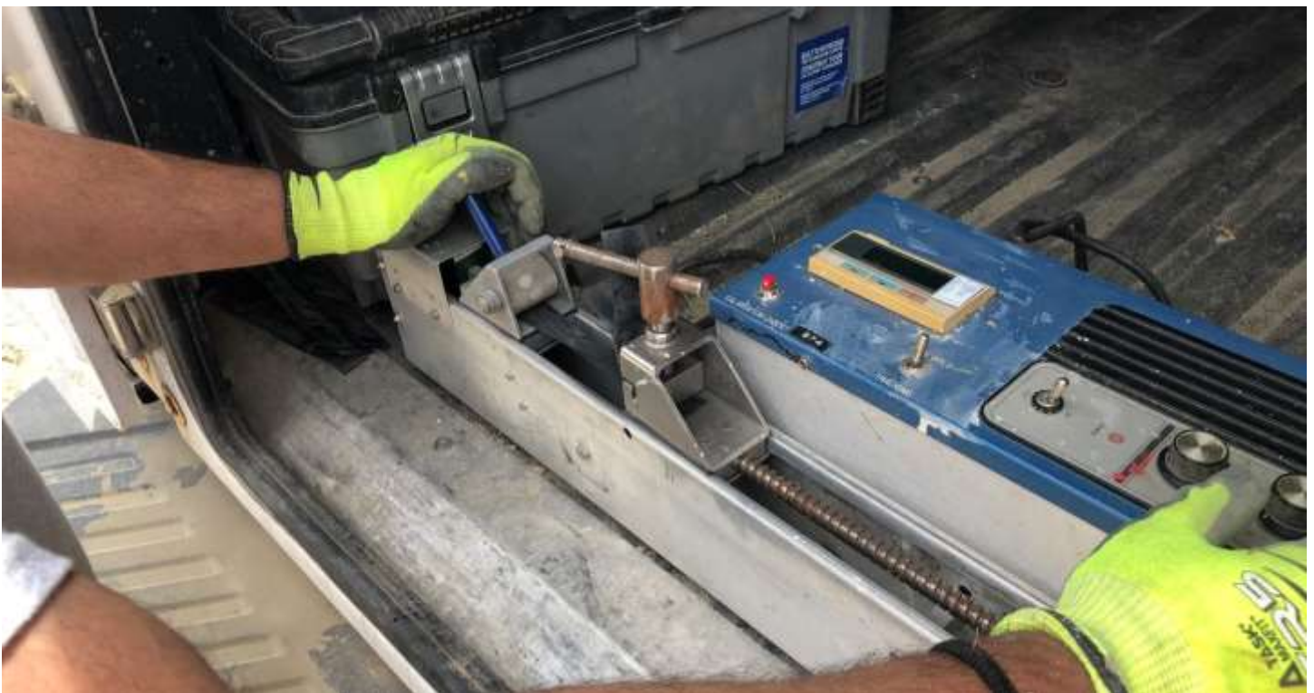
Picture # 6: WTL using tensiometer to conduct peel and shear tests on wedge weld test strips. A total of five peel tests and 2 shear tests were performed on the wedge weld.
