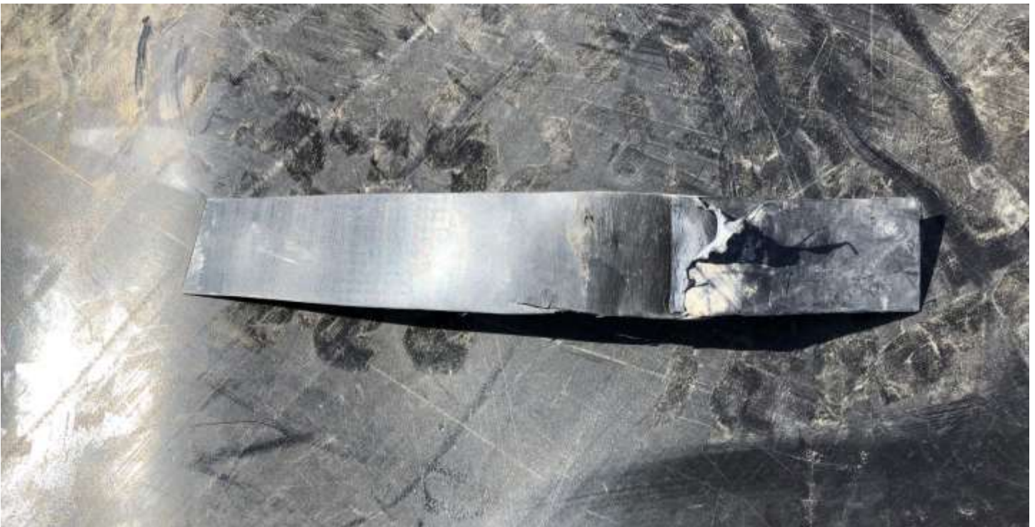
Picture # 6: Example of failed extrusion weld. WTL re-qualified the extrusion welder and re-sampled.
