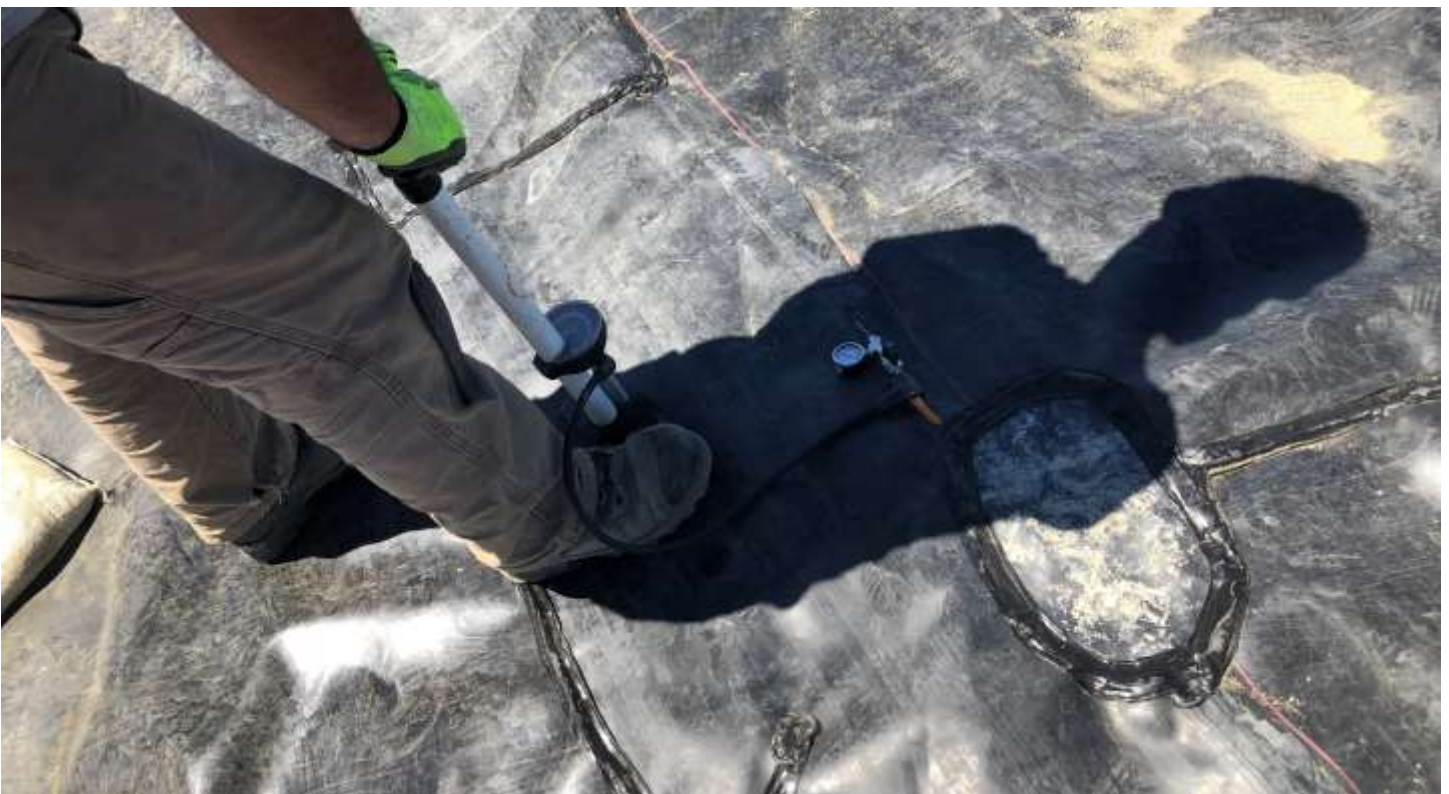
Picture #6: WTL air testing wedge weld.
