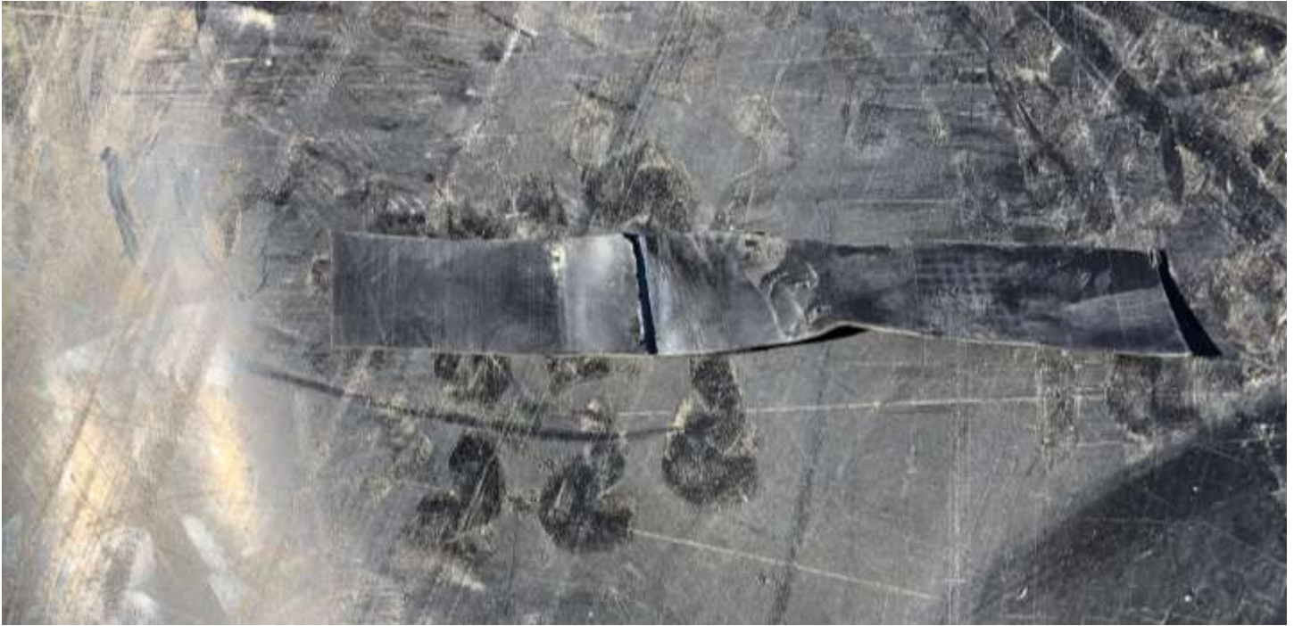
Picture # 7: Example of passed extrusion weld sample.
