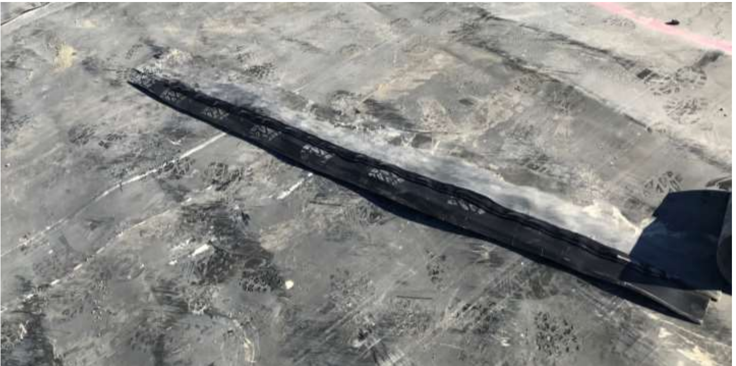
Picture # 2: Extrusion weld test strip.
