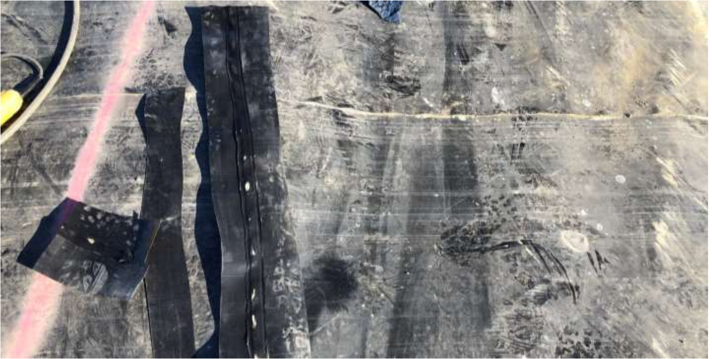
Picture # 1: Extrusion weld test sample.
