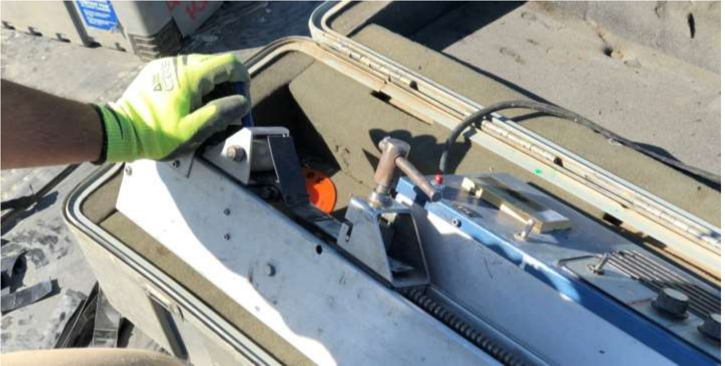
Picture # 5: WTL using tensiometer to test extrusion weld samples.
