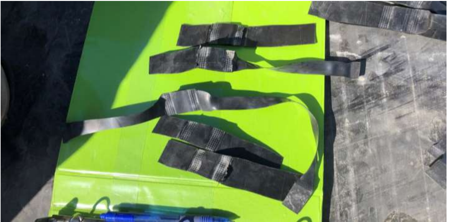
Picture # 3: Wedge weld samples passed.
