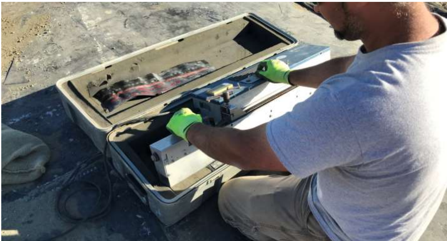
Picture # 3: WTL using tensiometer to test wedge weld and extrusion weld samples.
