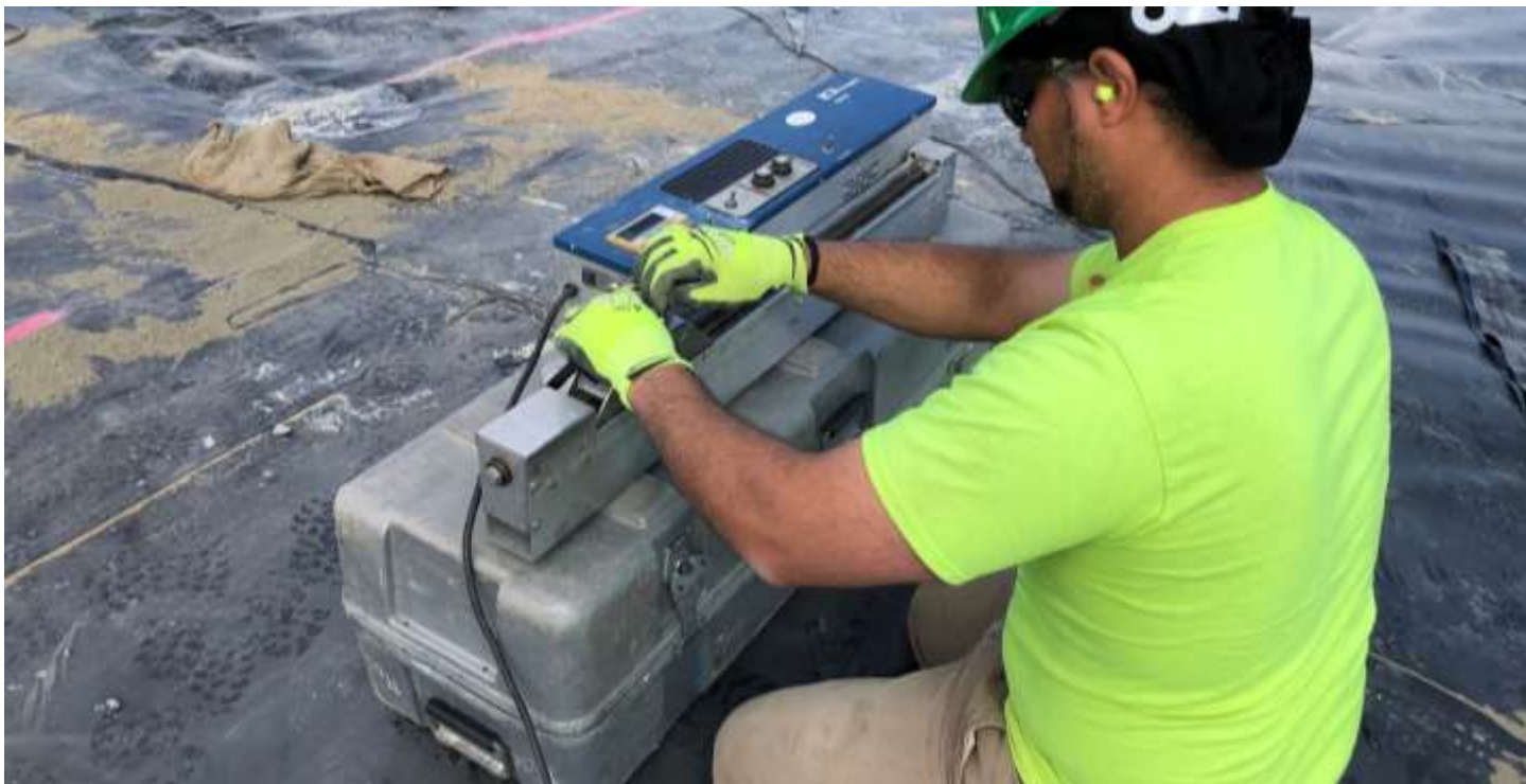
Picture # 1: WTL using tensiometer to test wedge weld.
