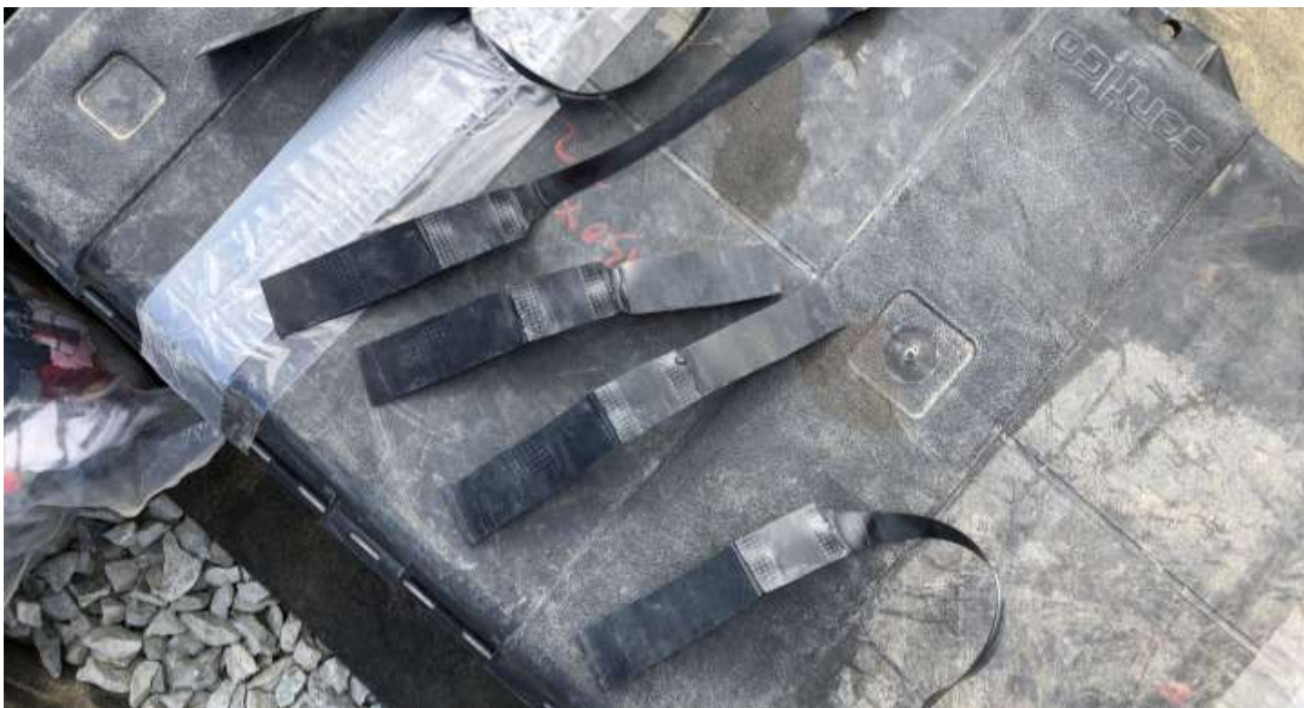
Picture # 2: Examples of passed wedge weld test strips.
