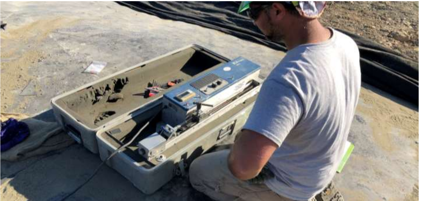
Picture # 2: WTL using tensiometer to test extrusion weld samples. A total of 5 peel tests and 2 shear tests were performed.
