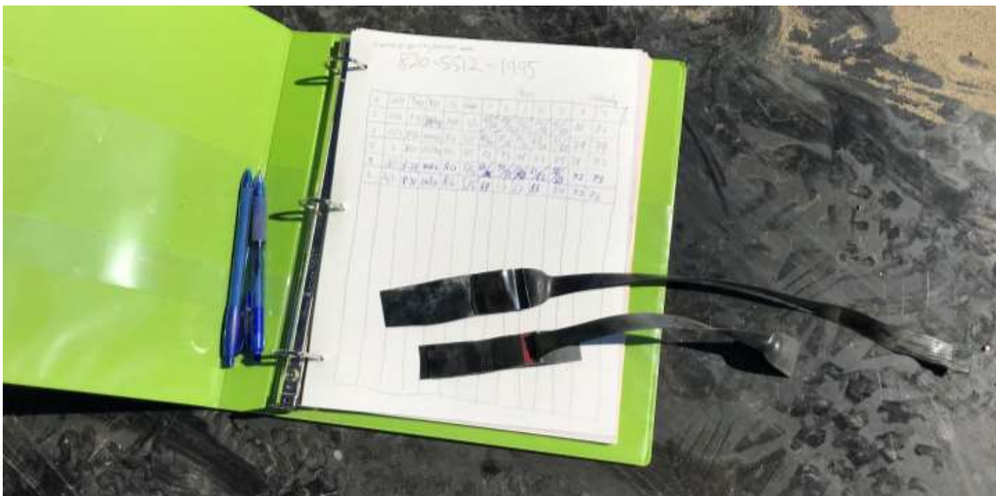
Picture # 4: Example of passed wedge weld and extrusion weld samples.
