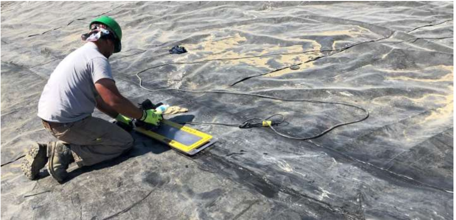
Picture #11: WTL performing vacuum box test on extrusion weld.
