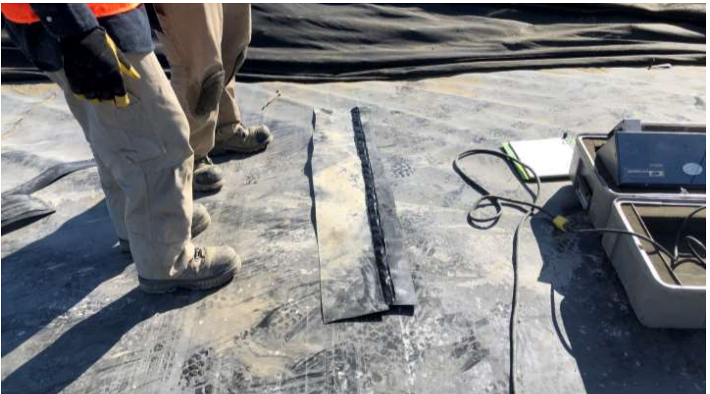
Picture # 4: WTL qualifying extrusion welder.
