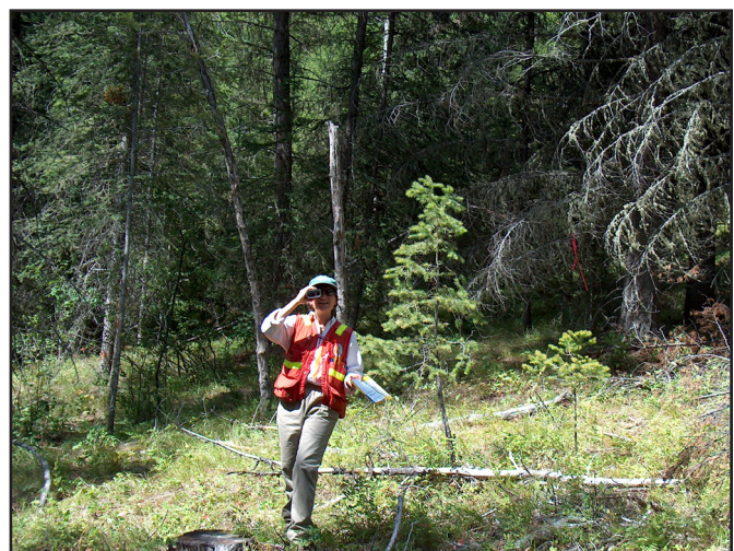
Measuring tree heights using laser range finder, Central Cariboo.
