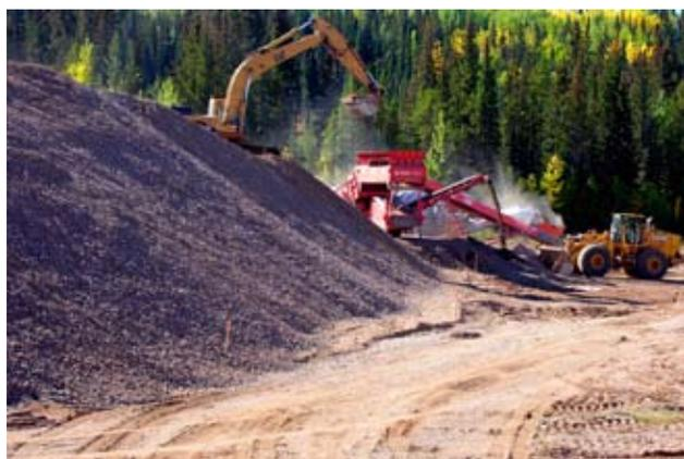
**Figure 6. Photograph of summer 2005 mining and processing activities at Kimea deposit. View towards the south, with the south side of Kimea Creek valley in the background.**
