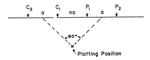
$C_1$  -  $C_2$  represents current dipole, length "a";  $P_1$  -  $P_2$  represents potential (measurement) dipole, length "a". Inter-dipole distance "na" is increased to provide larger volumetric sampling of the measured media.
