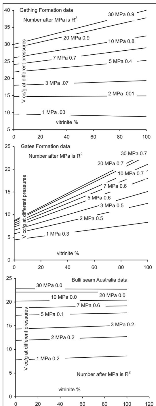
Figure 10. Effect of increasing pressure on vitrinite and inertinite adsorption with R<sup>2</sup> correlation factors for lines. Data from this study, Lamberson and Bustin, (1993) and Bustin *et al.* (1995).
