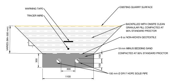
TYPICAL TWIN LEACHATE/LEAK DETECTION **CONVEYANCE PIPE TRENCH SECTION**
