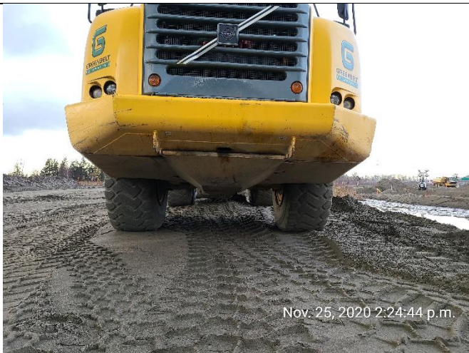
Photo 29. Drip trays had not been placed under all idle equipment, despite being readily available.
