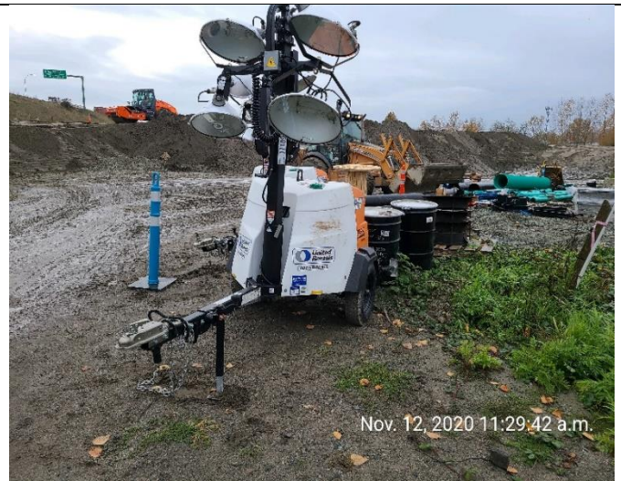
Photo 28. Some equipment such as light stands were lacking secondary containment.
