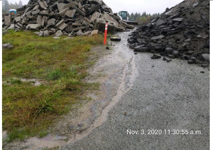
Photo 24. A hydrocarbon sheen was leaching from the asphalt stockpile at Area G.
