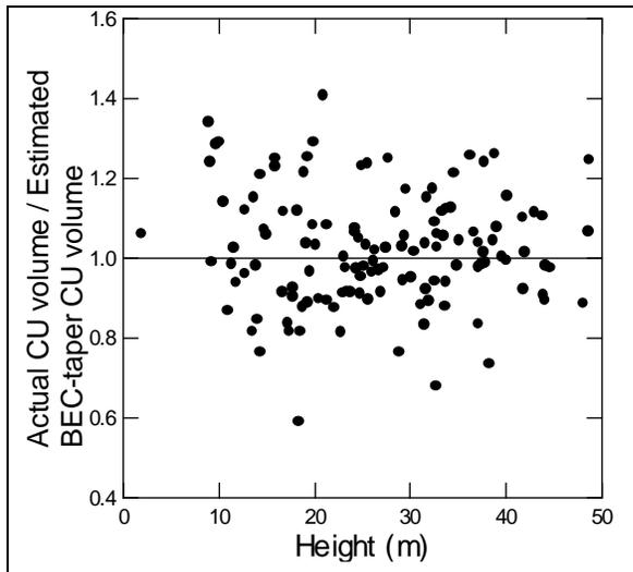
Figure 7: BEC-based taper equation bias for individual samples, as a function of tree height.
