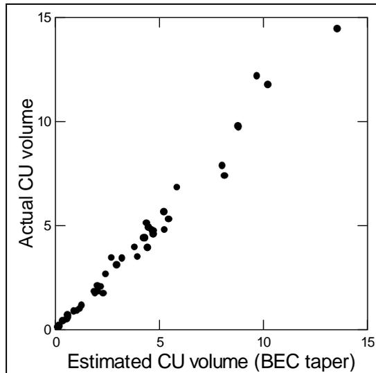
Figure 20: Relationship between actual CU volume from destructive sampling and CU volume estimated using BEC-based taper equations, for hemlock.
