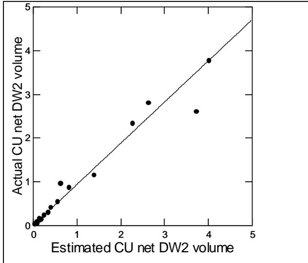
Fig. C-13: Immature (all species) stratum – actual CU net DW2 volume vs. BEC-taper net factored CU net DW2 estimated volume. Line indicates the NVAF ratio.
