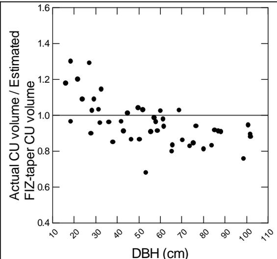
Figure D-32: FIZ-based taper equation bias vs dbh.
