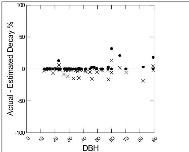
Figure 13: Bias in estimates of decay % for net factoring and loss factors, by dbh, for RISK GROUP 1. NOTE: ●'s represent net factoring bias and ×'s represent loss factor bias.
