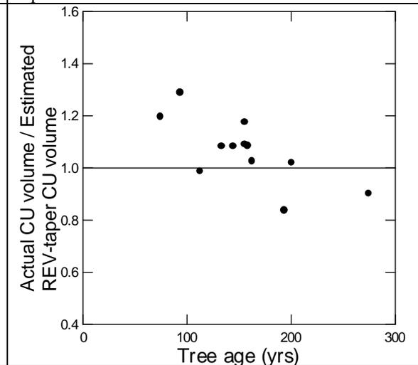
Figure D-27: Revenue Branch FIZ-based taper equation bias vs tree age.
