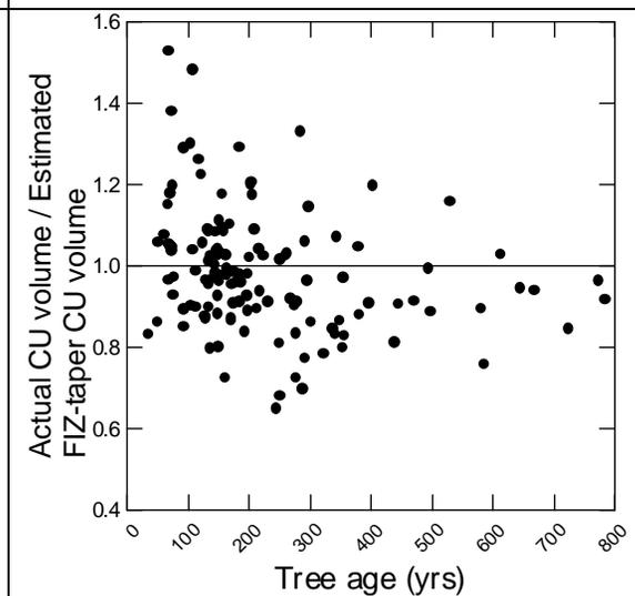
Figure 5: FIZ-based taper equation bias for individual samples, as a function of tree age.
