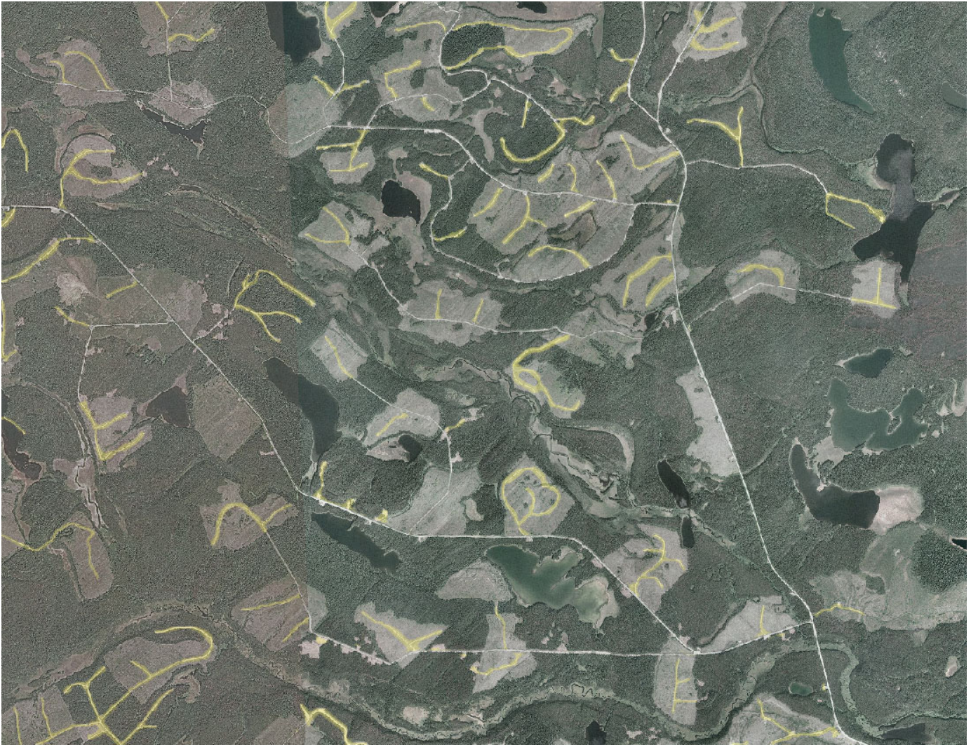
Figure 1: This aerial photograph, covering approximately 8500 hectares of intensively harvested low-relief terrain in northern BC, shows unrehabilitated TAS in yellow. The photograph shows 90% of cutblocks contained unrehabilitated TAS (generally roads), this TAS accounted for 1.4% of the overall area and 4.2% of the cutblock area. At this scale, the cumulative effect of accelerated drainage from these roads and the permanent access shown in white, could be significant.
