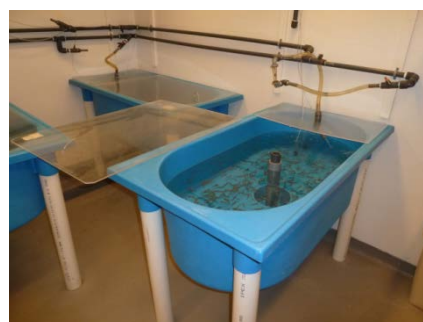
Figure 4: Example of a LC50 acute toxicity fish bioassay test using effluent ENV 2017
