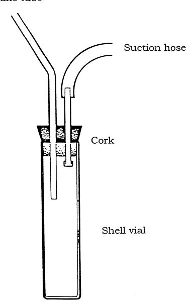
Figure 7. A mouth-operated vial aspirator (from Martin 1977).
