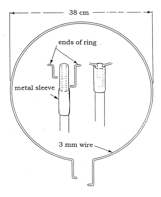
Figure 10. Details of insect sweep net, showing detachable wire ring and attachment to handle (from Martin 1977).
