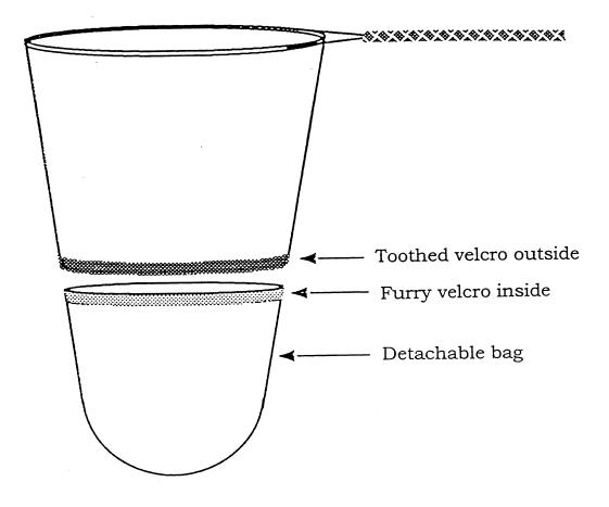
Figure 11. Diagram of sweep net showing detachable bag (from Milne 1993).
