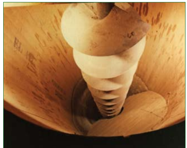
Figure 35. Close-up of the Danish auger dewinger.
