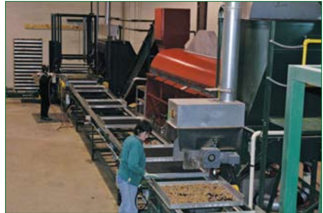
Figure 4. Christina Herman loading cones onto trays for kilning.
