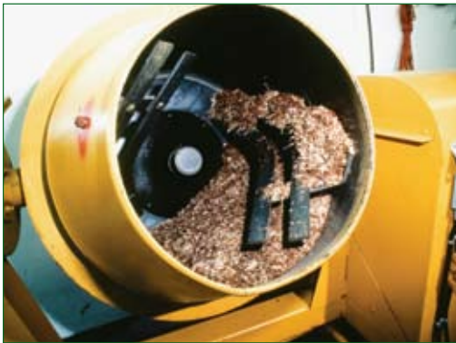
Figure 40. Large cement mixer dewinger. Duncan 1980.
