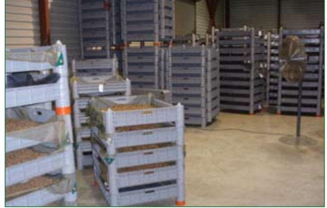
Figure 34. Abies cones stored on stacking plastic trays with additional aeration supplied by fans to assist in drying.
