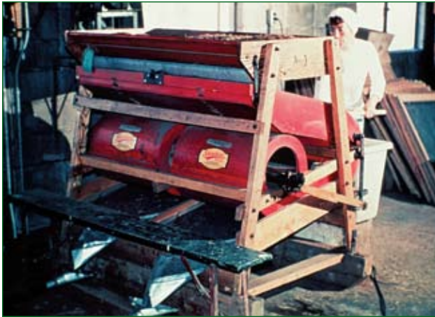
Figure 36. Standard Fanning mill screener with vacuum dewinger attachment.
