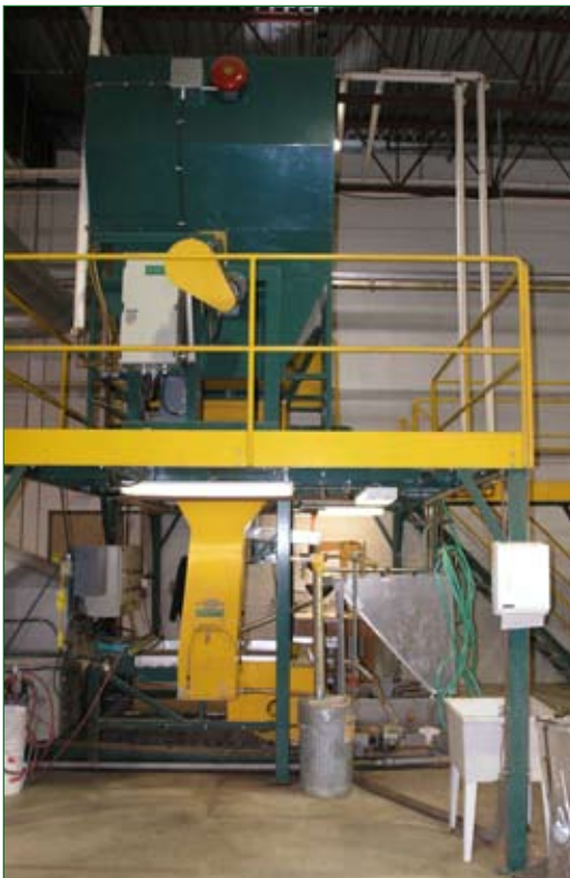
Figure 41. The Hilleshog /BCC Dewinger on the platform and aluminum liquid separation tank below at the Tree Seed Centre Surrey.
