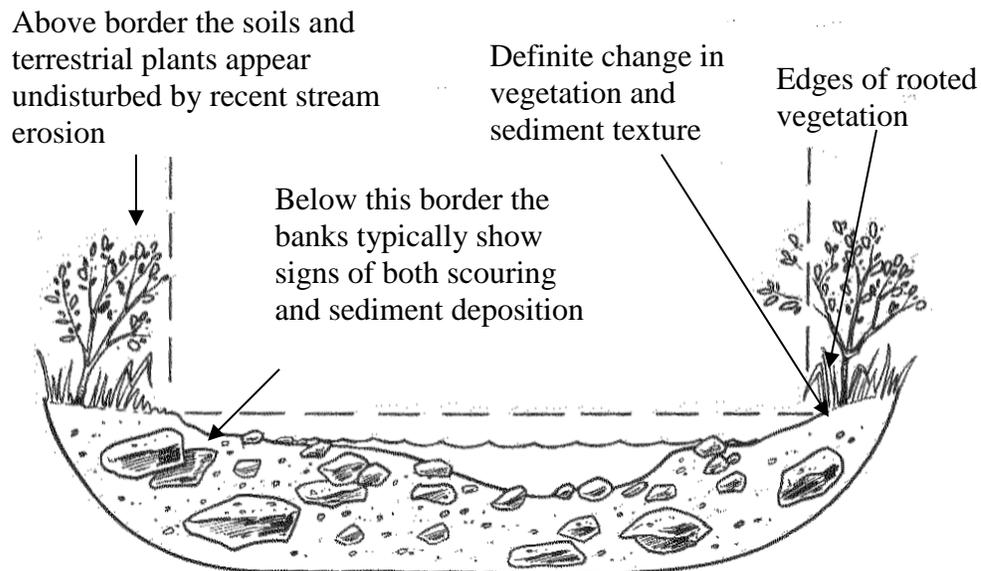
**Figure 3-2. Indicators of Bank-full Width for Streams**
