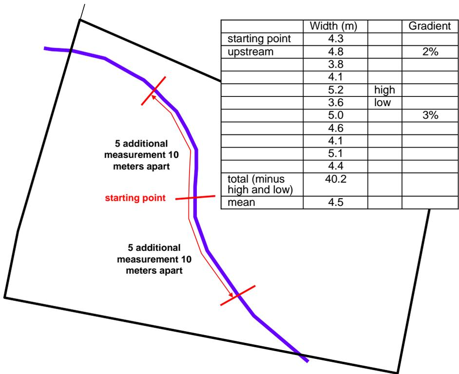
Figure 3-3: Calculating average channel width and channel slope
