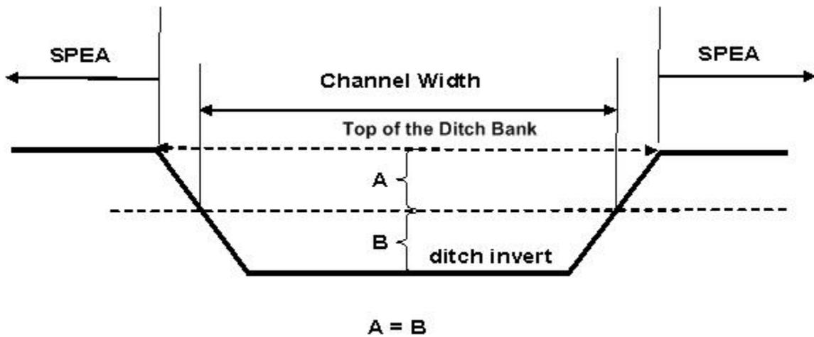
Figure 3-14: Determining Channel width for a Constructed Ditch
