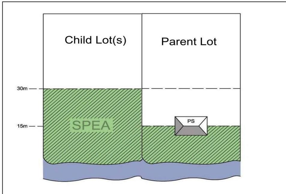
**Figure 2-4 Example of Wide Lot Scenario. The SPEA is reduced only on the Parent Lot based on the original Permanent Structure Child lots where there are no permanent structures have the maximum SPEA width for their Vegetation Category/Fish Bearing Status.**
