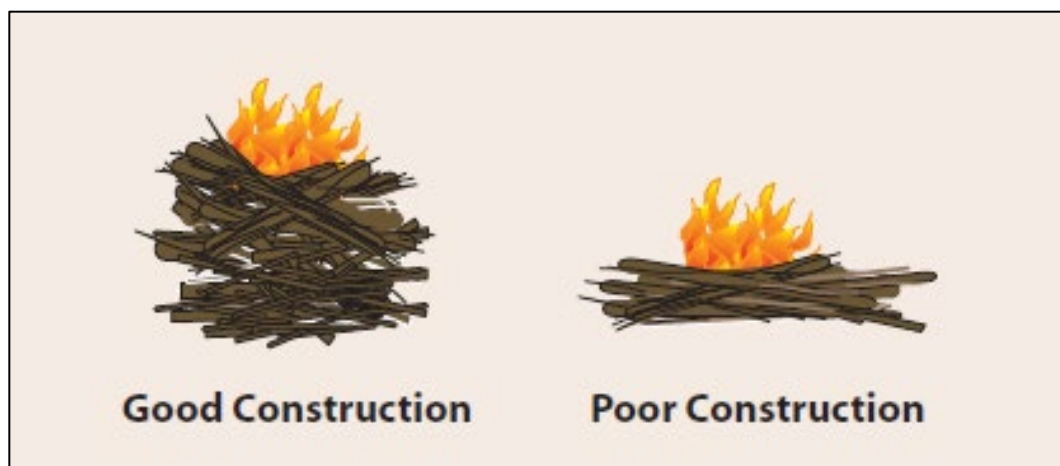
Figure 1. An example of good and poor pile construction. The good construction pile is stacked vertically with fine fuels at the bottom, covered with larger logs, for ease of ignition and optimal heat transfer. The poor construction pile is horizontal and has mixed fuel sizes at the base of the pile, leading to poor heat transfer.
