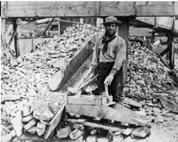
The rocker was an improvement on panning. The material was scooped into the rocker and washed over wooden strips to catch the heavier gold which sank to the bottom. A-00353
