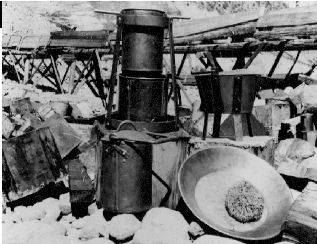
The goldpan and quicksilver (mercury) were the main tools for panning gold. The quicksilver attracted gold and when heated joined gold flecks together. G-00121
