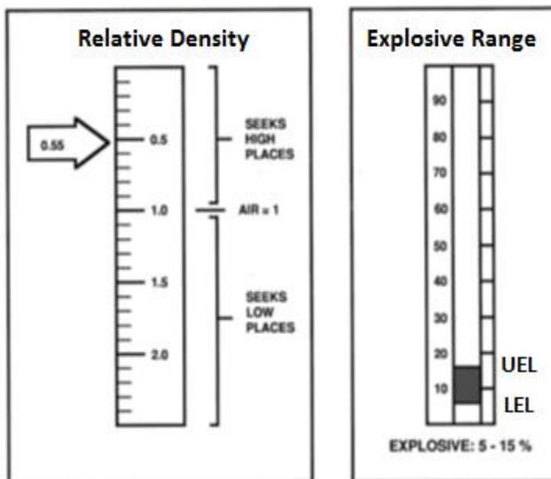
Fig 5.1 Relative density and Explosive range for Methane
