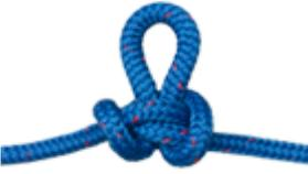
A blue rope tied in a butterfly knot, creating a loop in the standing part of the rope. |
