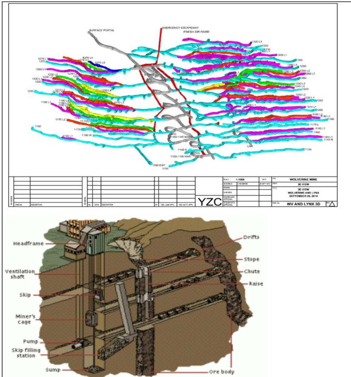
**Isometric drawings** are three-dimensional pictures of the mine workings. It shows what the workings would look like if all the rock surrounding the mine openings was transparent. With the advent of trackless mining methods using inclined and spiral ramps, normal mine drawings become quite difficult to read unless you are familiar with the mine layout, whereas isometric drawings provide a quick overview.
