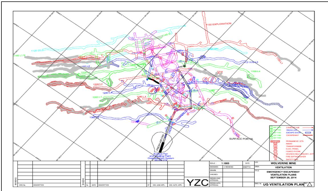
**Plan view mine drawings** provide an overhead view of a mine. Mines will have separate plans drawn for each level in the mine. They are drawn at various scales and the scale will always be noted on the drawing. A legend will be included to indicate the symbols used for fans, ventilation doors, shafts, raises, ore passes and so on. The symbols may vary from mine to mine.
