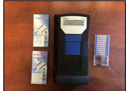
The chip has 10 individual sample tubes. Each tube can only be used once. The tester scans the chip when inserted into the reader and indicates the gas and range for which the chip is designed.
