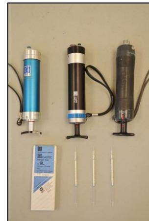
*Dräger (L) and Gastec (R) colorimetric tubes*
