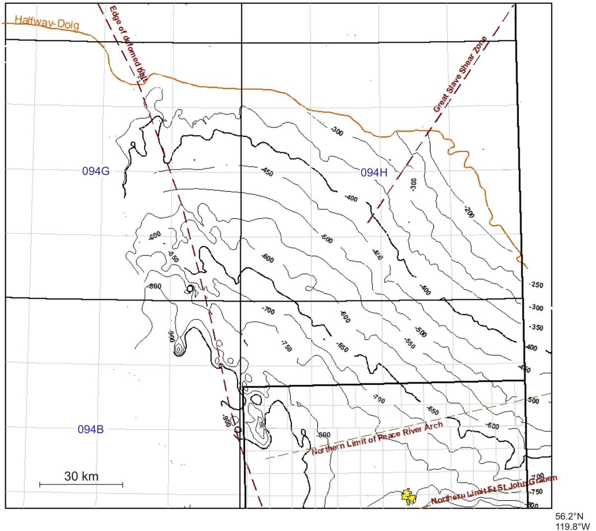
Figure 4. Structural elevation top of the Halfway Formation (contour interval 50 m): The Halfway Formation dips more or less uniformly to the southwest until the deformed belt, where the structure becomes more complex. The influence of deep-seated faulting might be evident by deviations from the general trend near the Fort St. John graben in the southeast.
