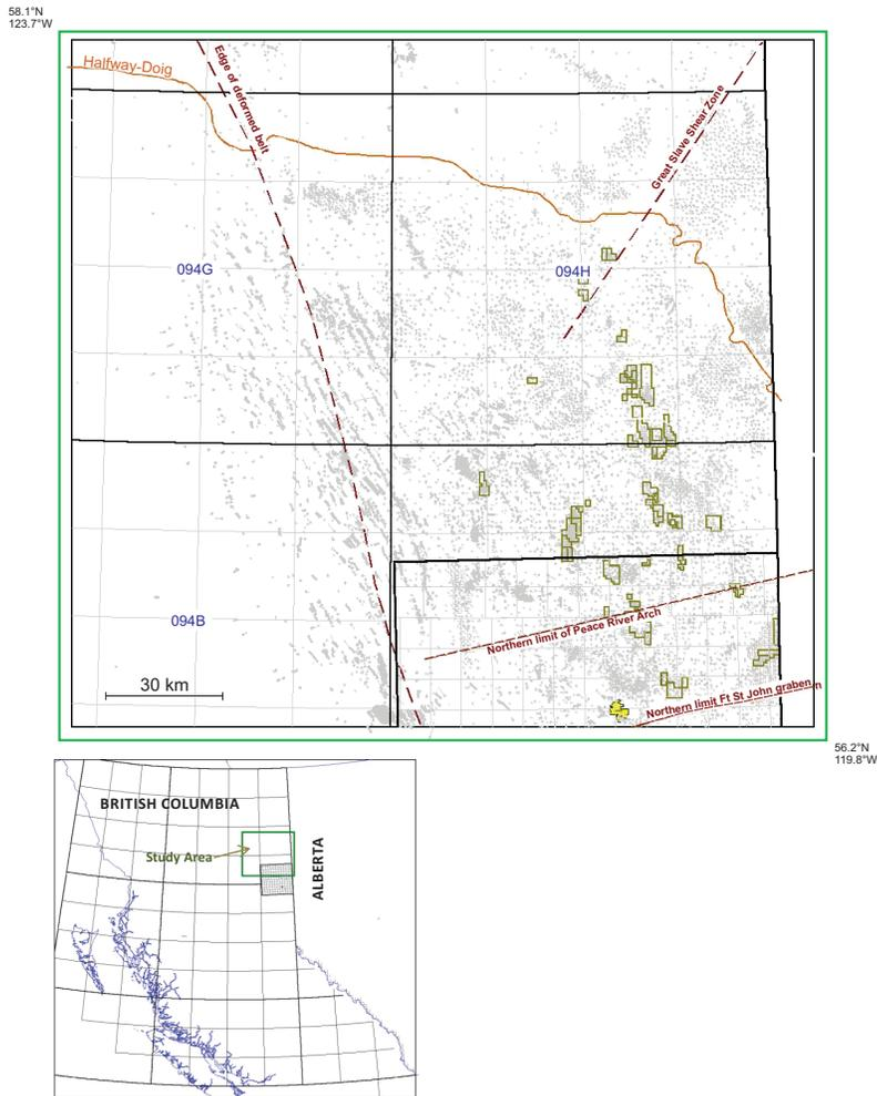
Figure 1. Study area: The Halfway Formation is constrained to the north-northeast by an erosional limit (brown line). To the west it thickens and the structure becomes more complex beyond the edge of the deformed belt. Green polygons represent the main oil-producing pools of the Halfway Formation; grey dots represent all wells within the study area.
