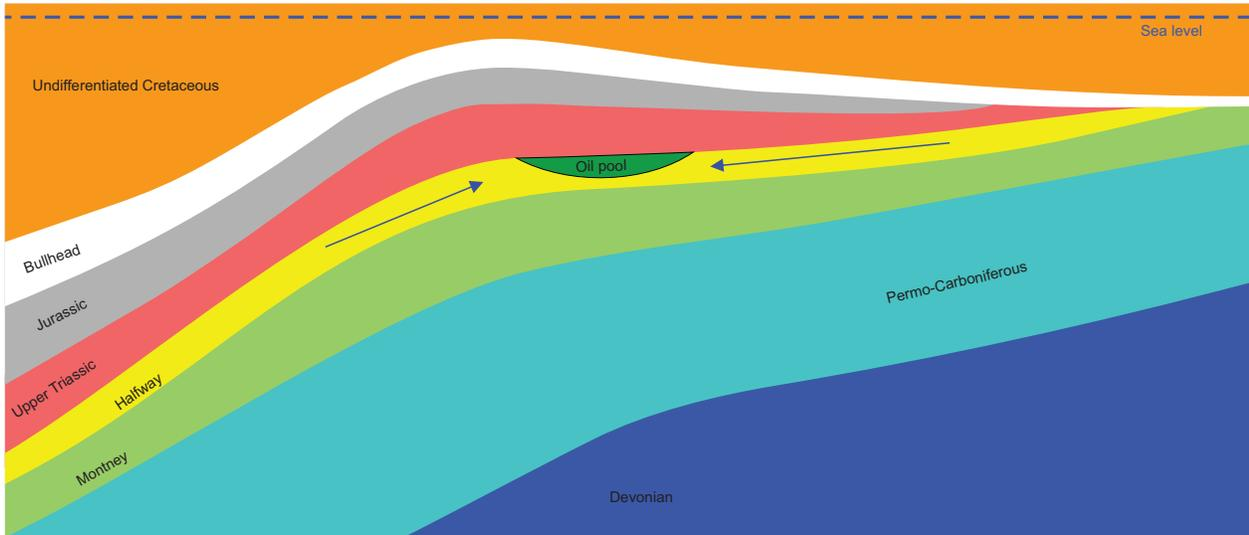
Figure 7. This schematic cross-section illustrates how the Halfway Formation comes up against the Bullhead aquifer to the east. Fresh recharge might take place along the edge. Hydrodynamic flow is mostly updip from west to east, except for a small reversal from the edge. The arrows show inferred direction of formation fluid flow and suggest a possible mechanism for oil entrapment approximately where flow is slowed in an area of lower potential.
