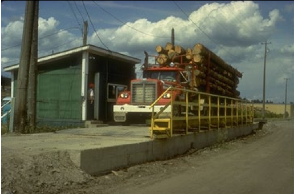
Figure 13.4 A Loaded Logging Truck on the Platform of a Weight Scale.
