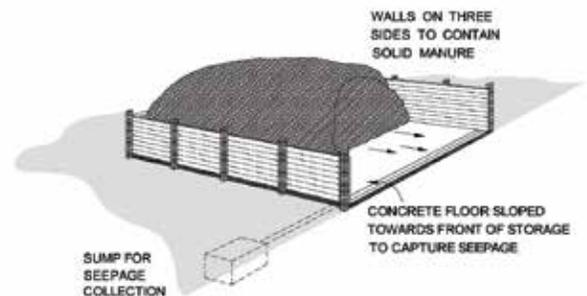
FIGURE 3.6 Typical Solid Manure Storage Facilities
