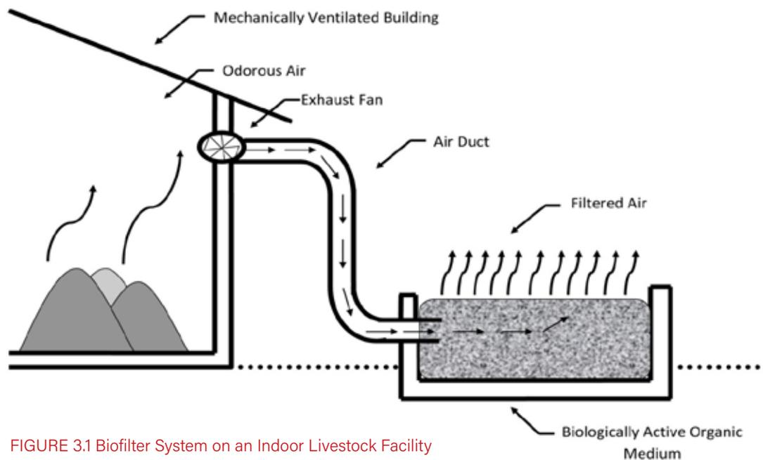
FIGURE 3.1 Biofilter System on an Indoor Livestock Facility
