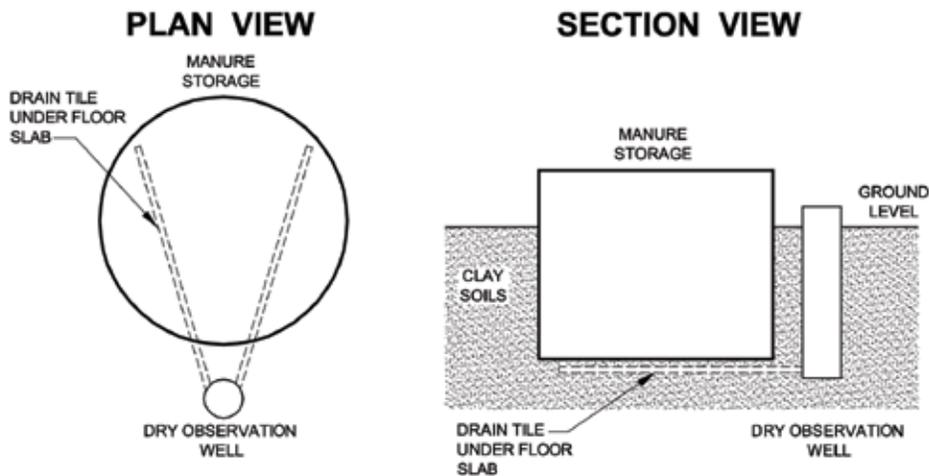
FIGURE 3.5 Leak Detection Under a Manure Storage Facility
