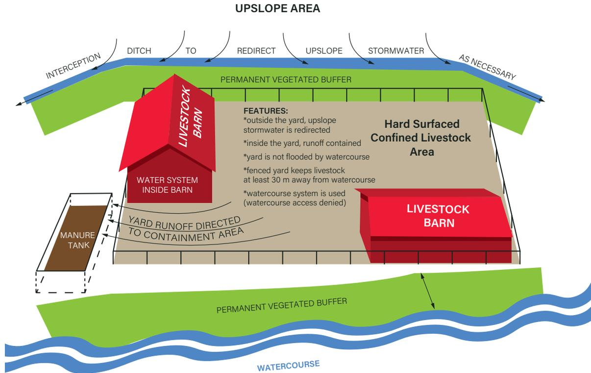
FIGURE 3.3 An Environmentally-Sound Confined Livestock Area – Hard-Surfaced Yard
