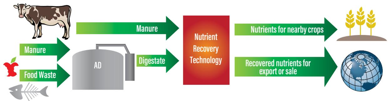
FIGURE 3.7 Nutrient recovery process on the farm (Source: Hallbar Consulting, 2016).
