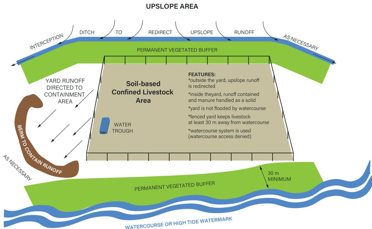
**FIGURE 3.2 An Environmentally-Sound Confined Livestock Area – Soil-Based Yard**
