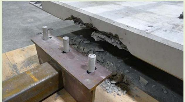
at failure, A325 bolts
