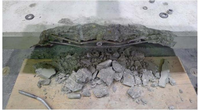
Figure 58: Steel post, Test #3.4, horizontal load component applied, 2 x 2 x A307 horizontal bolts
