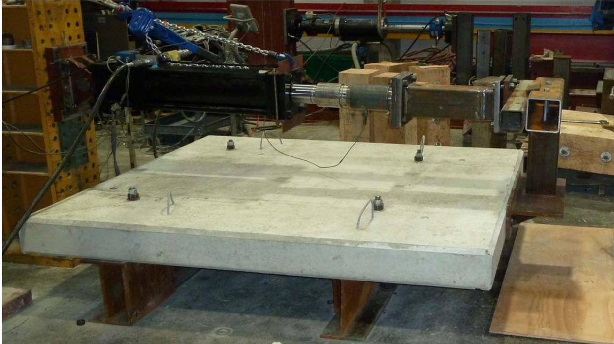
Figure 46: Steel post, Test #2.11, 3 x A325 horizontal bolts
