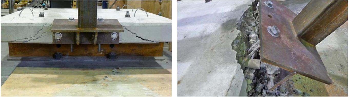
Figure 52: Steel post, Test #3.1, vertical and horizontal load components applied, 2 x 2 x A307 horizontal bolts
