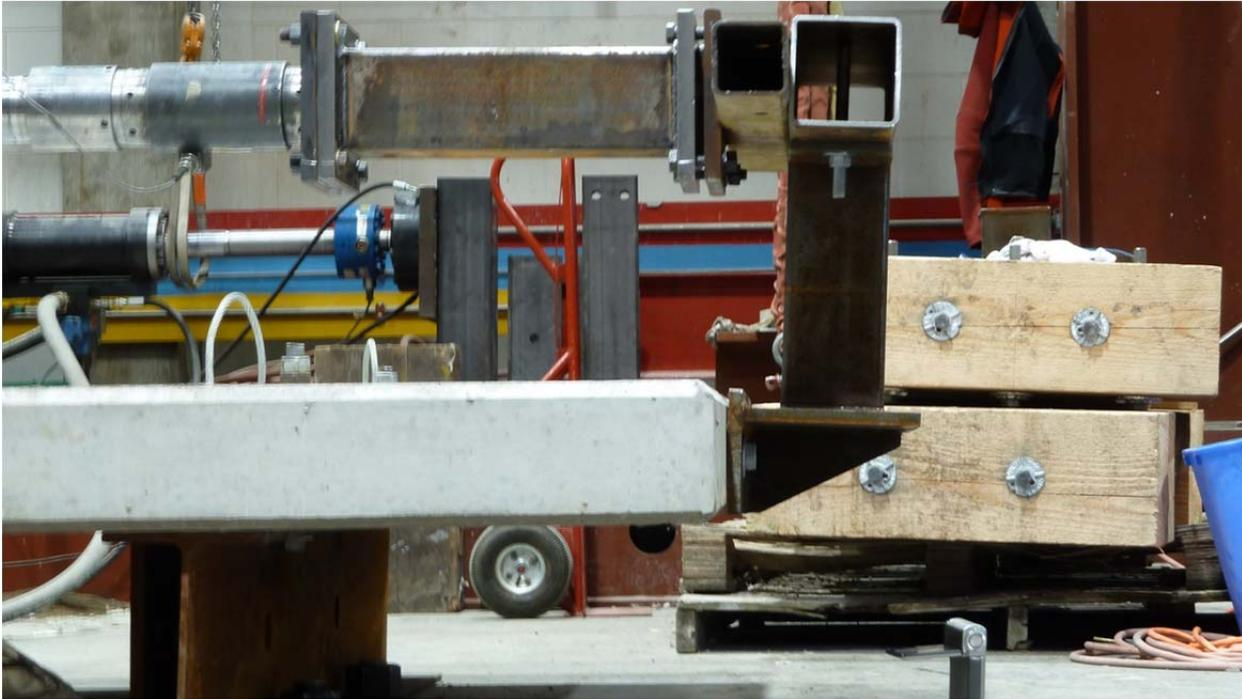
Figure 40: Steel post, Test #2.2, 3 x A307 horizontal bolts
