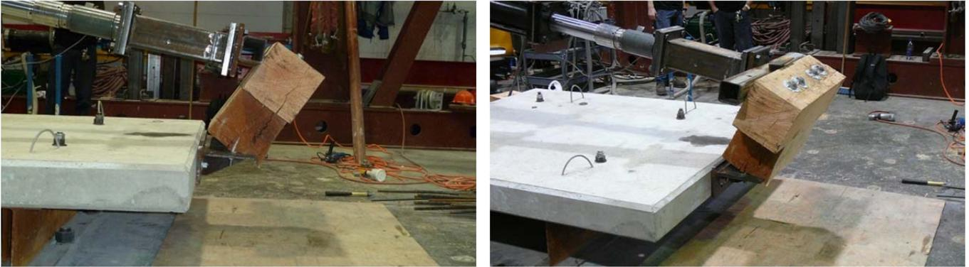
Figure 62: Steel post, Test #4.2, steel base, timber riser, vertical and horizontal components applied, 3 x A307 horizontal bolts
