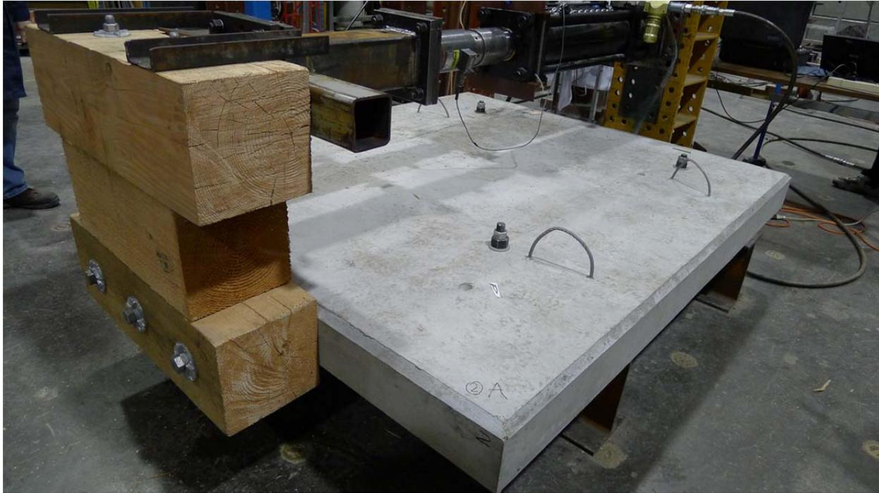
Figure 28: Timber curb block, Test #1.2
