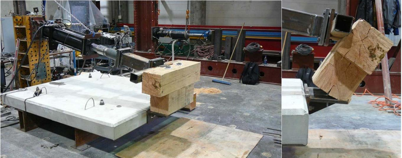
Figure 60: Steel post, Test #4.1, steel base, timber riser, vert. and hor. components applied, 3 A307 horizontal bolts
