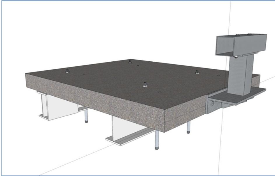
Figure 9: 3-D view of set-up for steel post curb attachment
