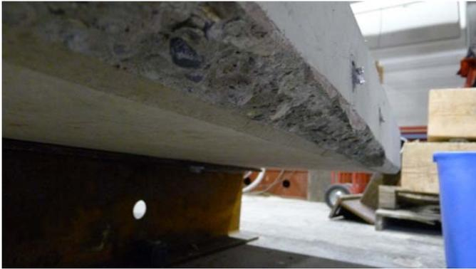
Figure 39: Concrete deck edge, spalled material limited by drip groove, Note: highlighted crack at midthickness of deck panel
