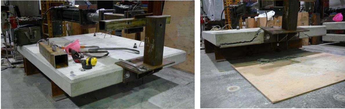
Figure 56: Steel post, Test #3.3, horizontal load component applied, 2 x 2 x A307 horizontal bolts
