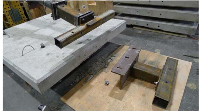
Figure 42: Steel post, Test #2.3, vertical and horizontal load components applied, 3 x A307 horizontal bolts
