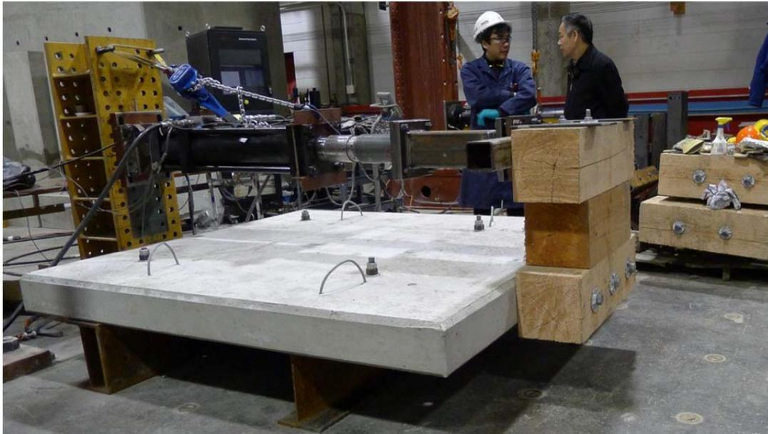
Figure 25: Timber curb block, Test #1.1, horizontal load direction
