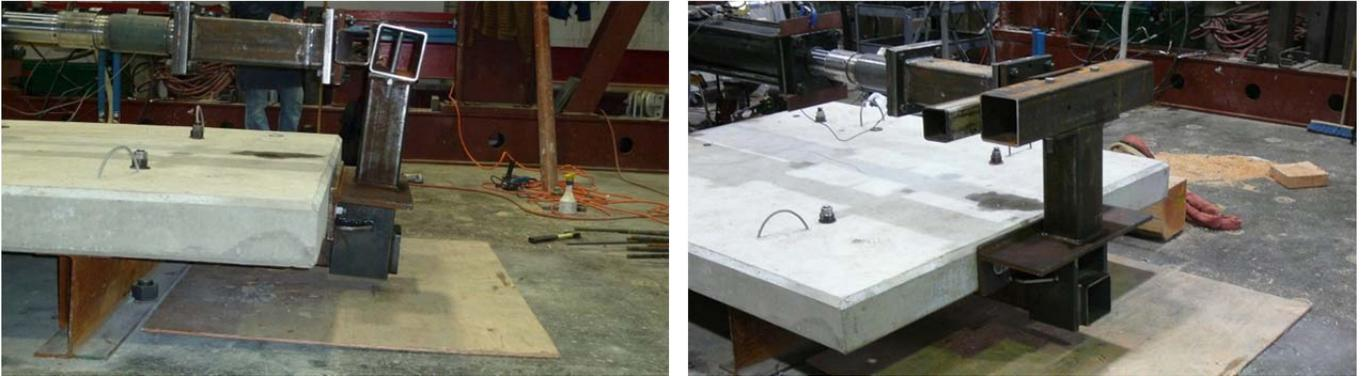
Figure 64: Steel post, Test #4.3, horizontal load, 3 x A307 horizontal bolts
