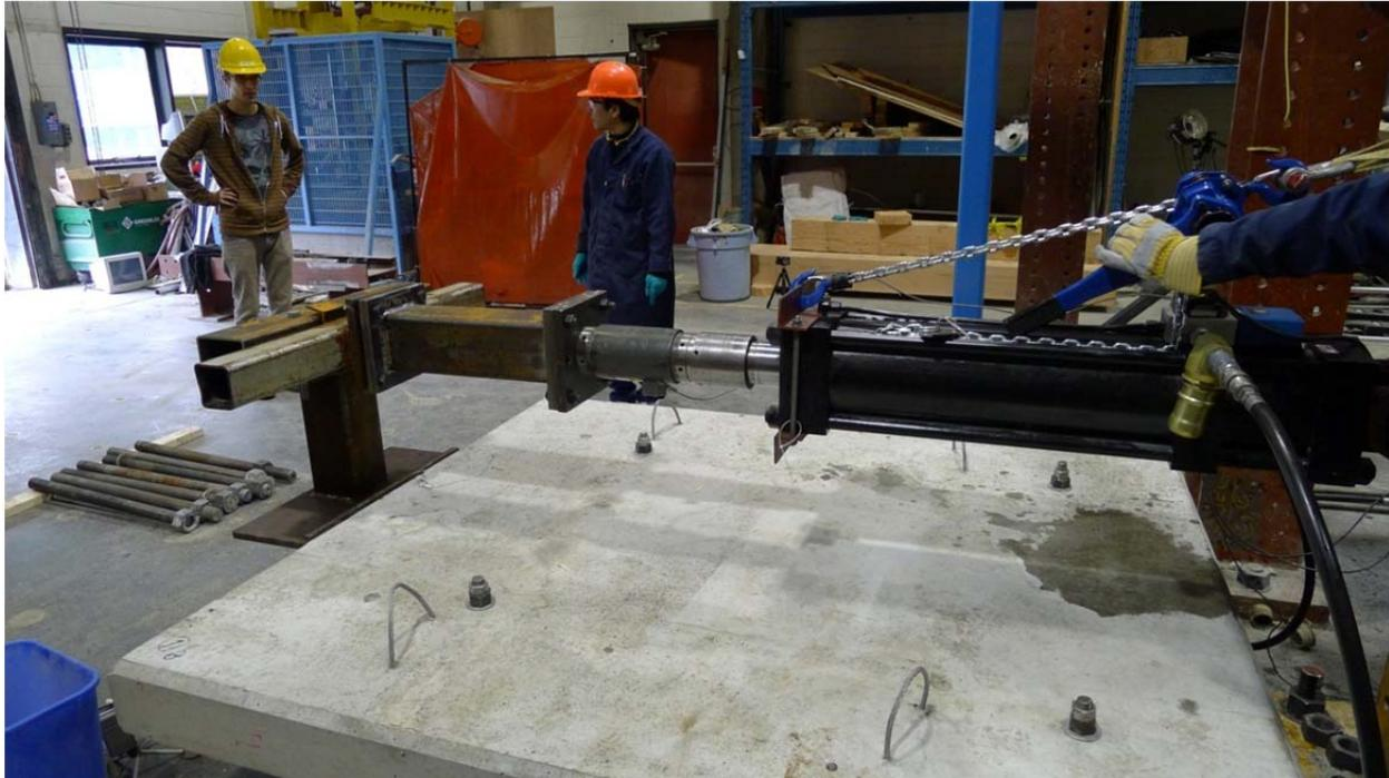
Figure 35: Steel post, Test #2.1, horizontal load direction, 3 x A307 horizontal bolts
