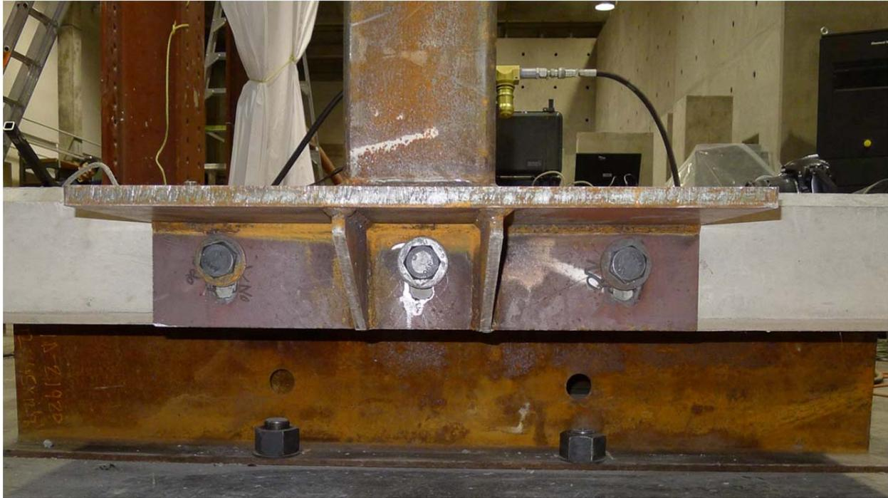
Figure 49: Steel post, Test #2.21, 3 x A325 horizontal bolts
