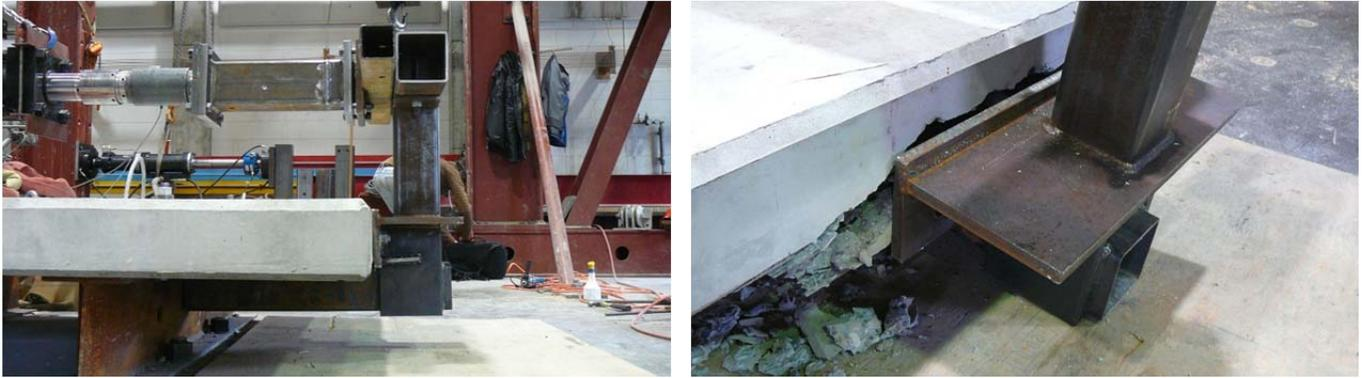
Figure 66: Steel post, Test #4.4, horizontal load, 3 x A307 horizontal bolts
