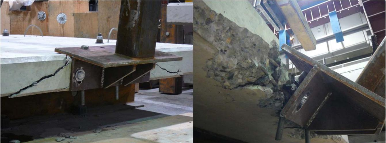
Figure 54: Steel post, Test #3.2, vertical and horizontal load components applied, 2 x 2 x A307 horizontal bolts
