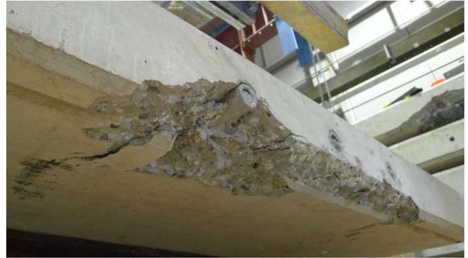
Figure 44: Steel post, Test #2.4, vertical and horizontal load components applied, 3 x A307 horizontal bolts
