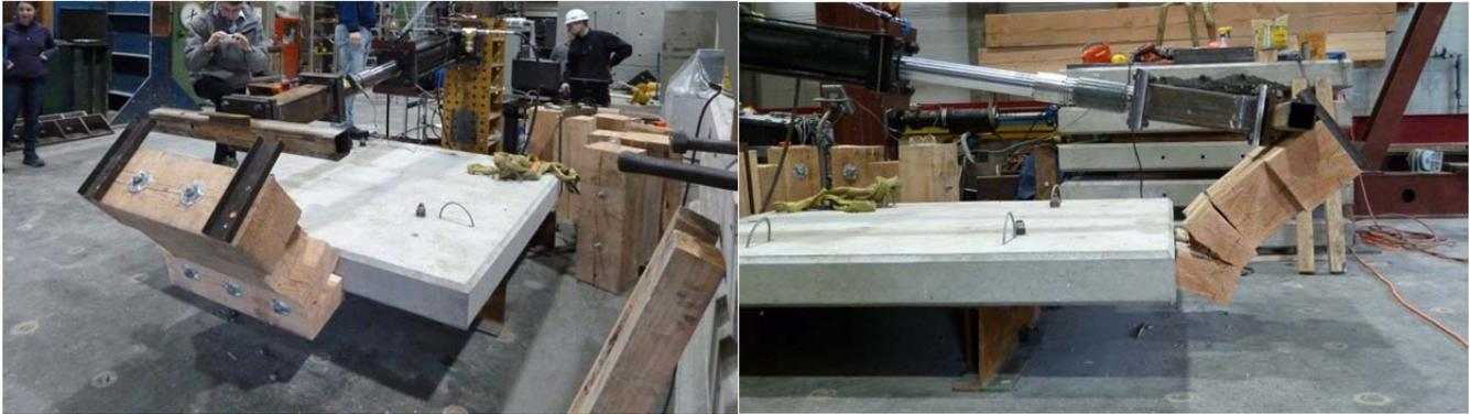
Figure 33: Test Series 1.4, horizontal and vertical load components applied
