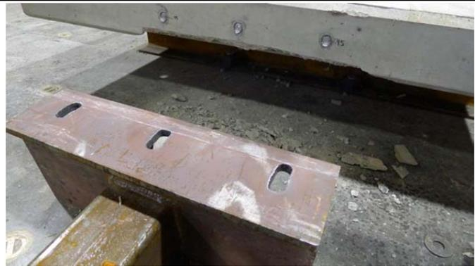
Figure 38: All three bolts stripped in tension, lower concrete face spalled
