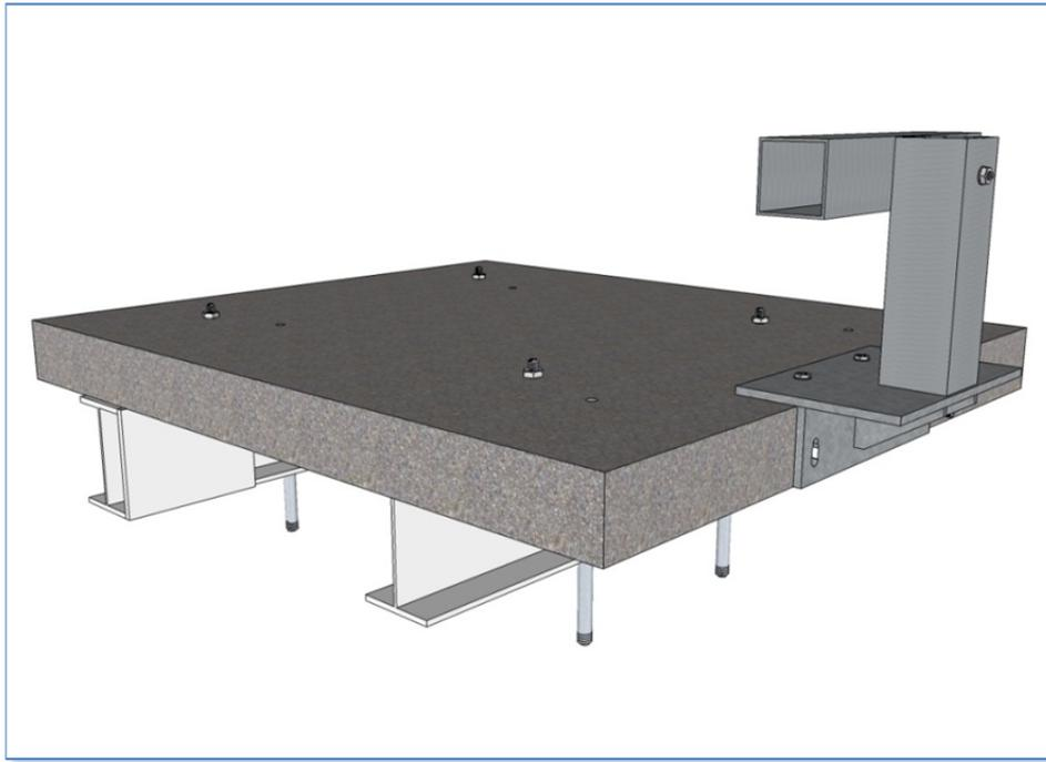
Figure 11: 3-D view of set-up for (modified) steel post curb attachment
