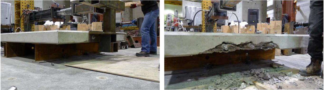
Figure 68: Steel post, Test #4.5, vertical load component applied, 3 x A307 horizontal bolts
