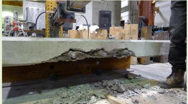
at failure, A307 bolts
