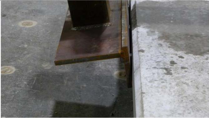
Figure 37: Note: Bolt elongation just before failure
