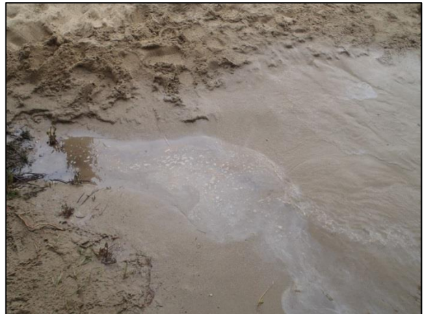
Photo 4. Section 2b (under ferry ramp) – silver to iridescent film observed when shoreline washed.
