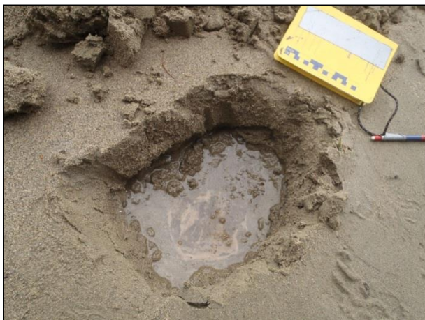
Photo 5. Section 2b – pit – no film or subsurface oil present
